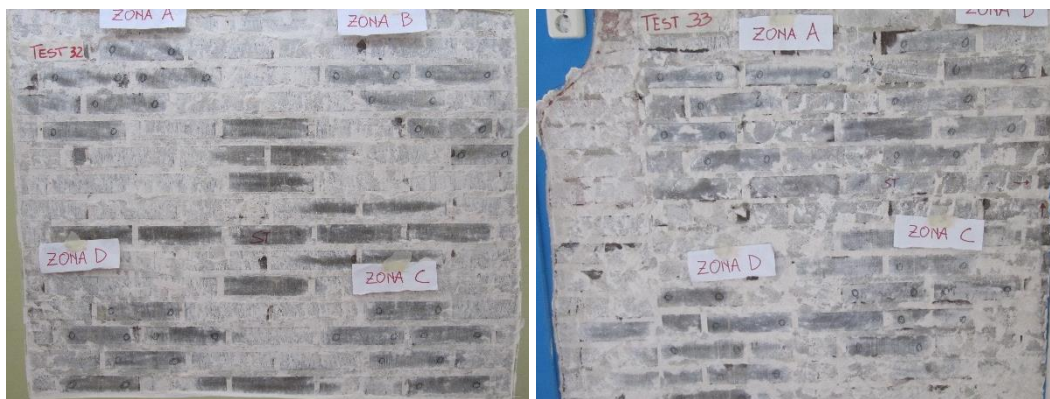
Figure 34. Example of Older Dark Good Quality masonry for the Clay > 1945 typology.
