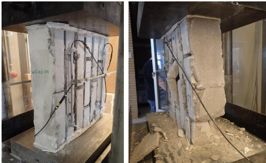
Figure 11. Horizontal Compression Test on Masonry Samples.
