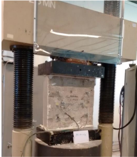
Figure 14. Vertical Compression Test on Masonry Samples.
