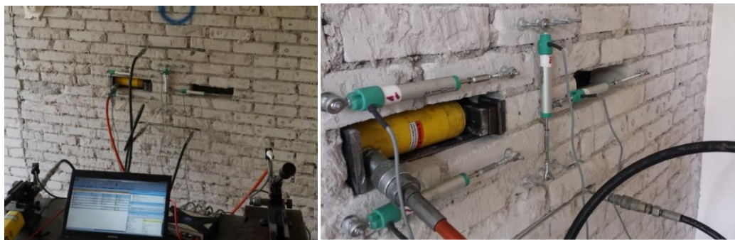
Figure 8. Shove Test: setup.
