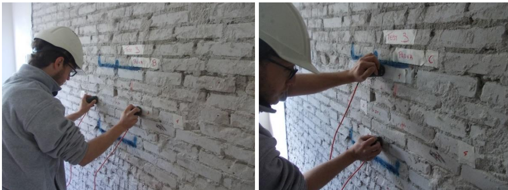
Figure 4. Ultrasonic Test: indirect horizontal configuration (left) and indirect vertical configuration (right).
