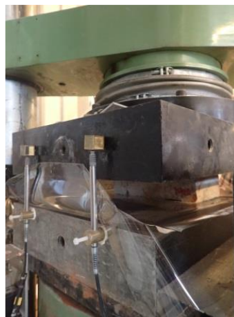
Figure 9. Compression Test on Masonry Unit.
