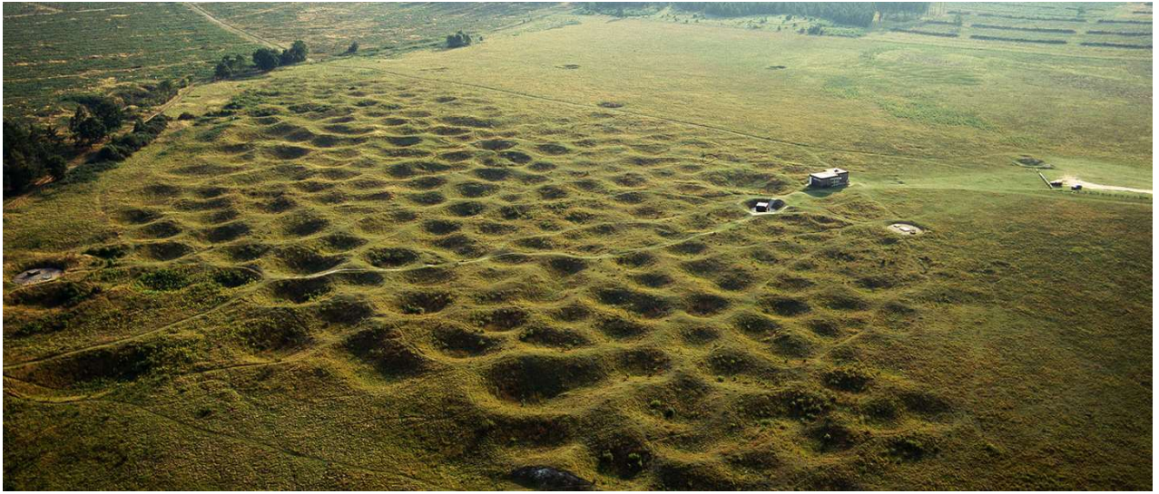
Figure 29: Aerial view of surface subsidence resulting from Neolithic flint mining at Grimes Graves, Suffolk, England 17 .
