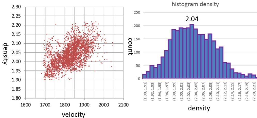
Figure 5: finding the density for the upper NS formation, using the information from logs from BRW-5 and ZRP-2. Since no clear relation exists between density and velocity, we take the value of 2.04 gr/cm<sup>3</sup>
