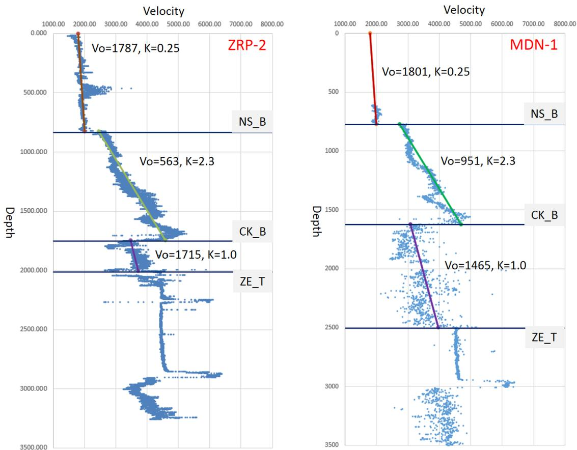
Figure 2: the velocity model of the Cenozoic and Mesozoic overburden until top Zechstein, plotted against the actual sonic logs of the wells ZRP-2 (on the left) and MDN-1 (on the right). Notice how well the velocity model captures the strong velocity increase at the NS\_B and the velocity inversion at the CK\_B, as well as the strong velocity increase in the Chalk layer, as expressed by the large  $K$  value of 2.3
