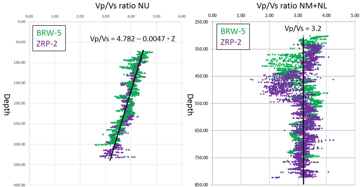
Figure 4: deriving the Vp/Vs ratios for the upper NS (left) and the lower NS (right) formations, based on the wells BRW-5 and ZRP-2. Note the depth dependency of the Vp/Vs ratio for the NU, as expressed by the formula, whereby Z stands for depth from surface.
