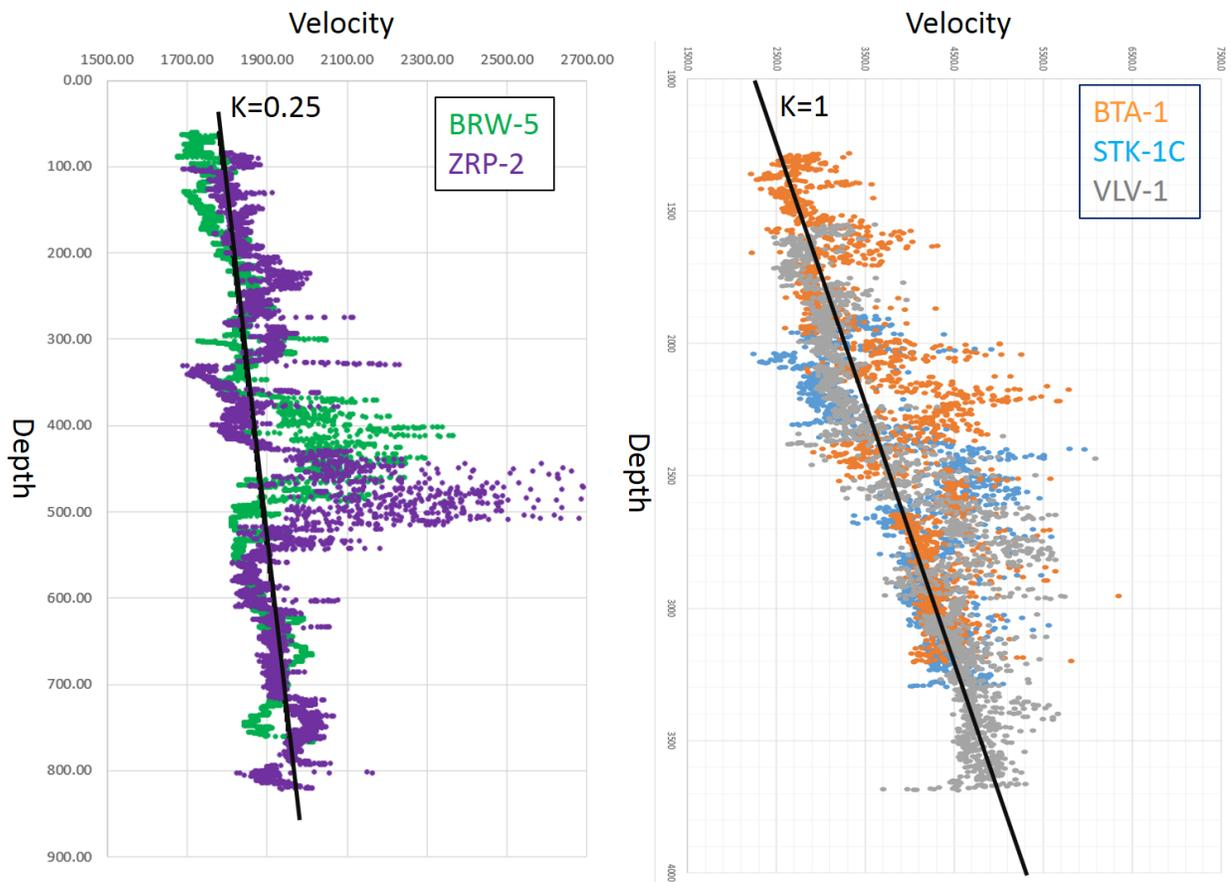
Figure 3: determining the K factor for the NS formation, based on the wells BRW-5 and ZRP-2, and for the Rijnland+Jurassic+Triassic formations, based on the wells BTA-1, STK-1C and VLV-1.
