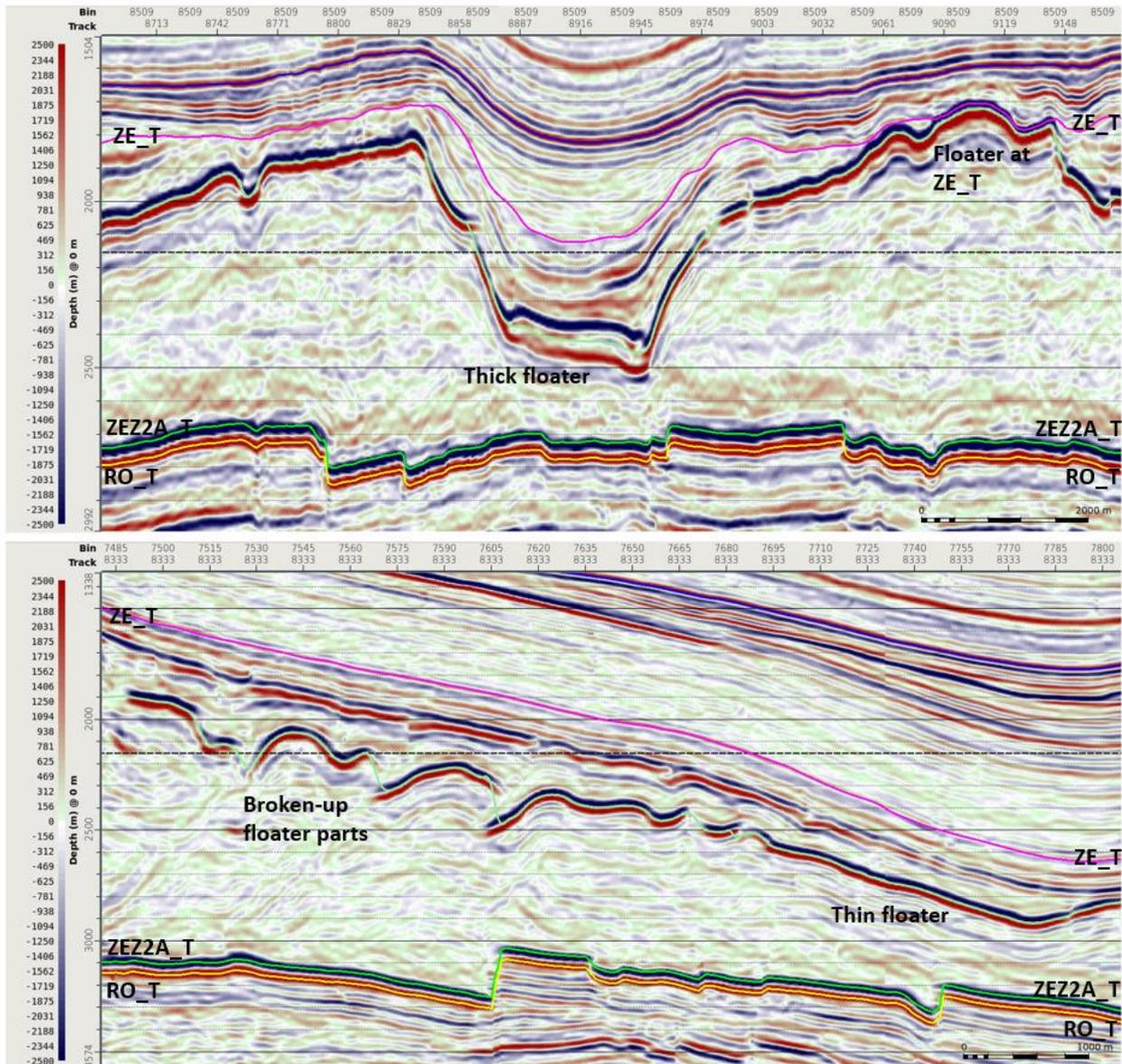
Figure 9: Various expressions of anhydrite/carbonate floaters in the Zechstein. Also shown is the 50 m thick basal anhydrite (ZEZ2A\_T) directly overlying the Rotliegend reservoir (RO\_T).
