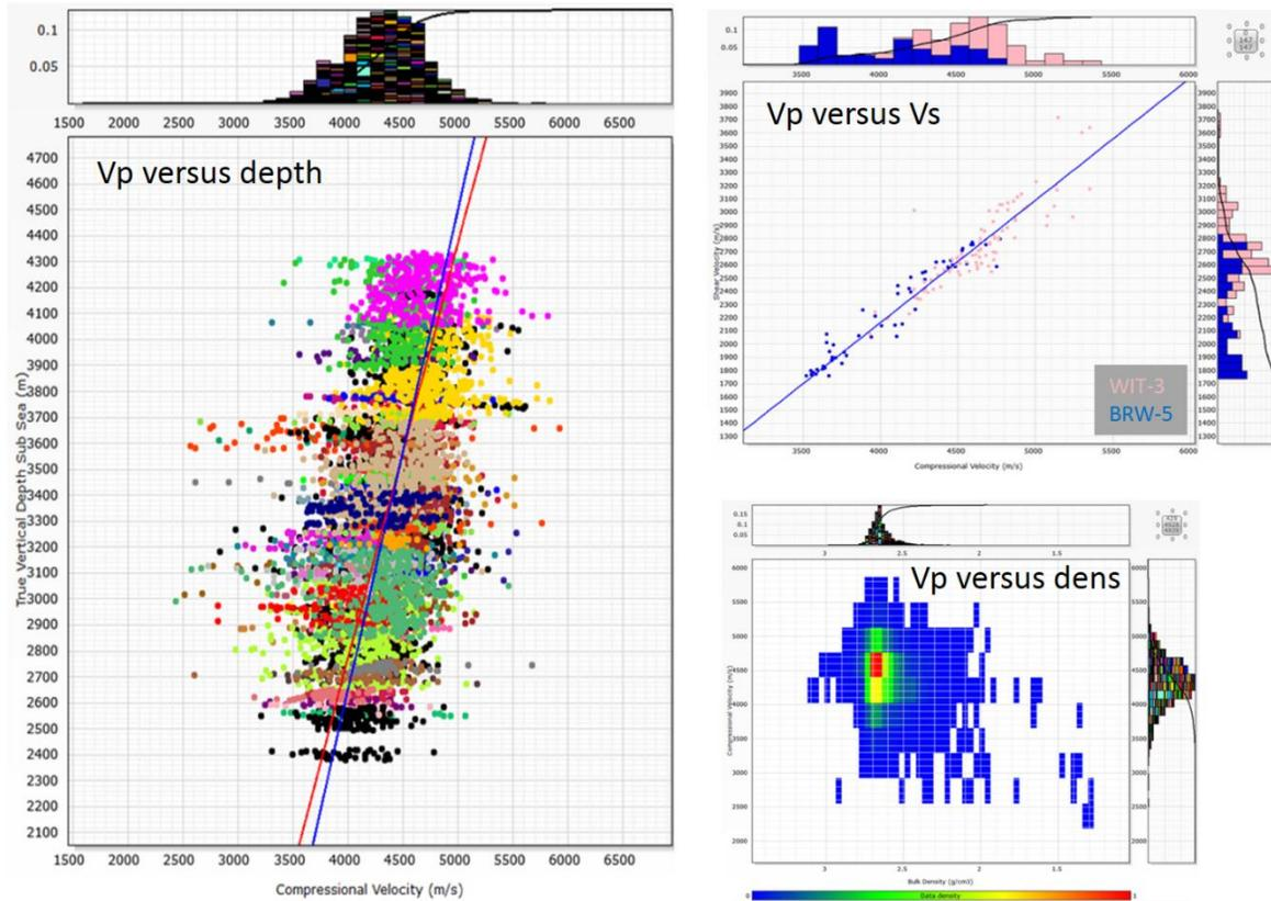
Figure 12: Carboniferous underburden. Left: Vp versus depth using multiple well logs, each indicated with a different color. The blue trendline is without outliers, the red one with outliers included. Top right: Vp-Vs relation. Bottom right: Vp versus density crossplot. The highest coexistence of density / velocity values, the red spot, at 2.65 gr/cm<sup>3</sup>
