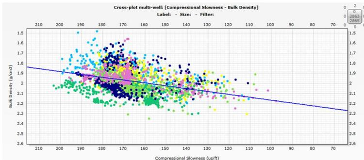
Figure 6: relation between density and P wave slowness for the lower NS formation. Multiple well logs were used, as indicated by the different colors.
