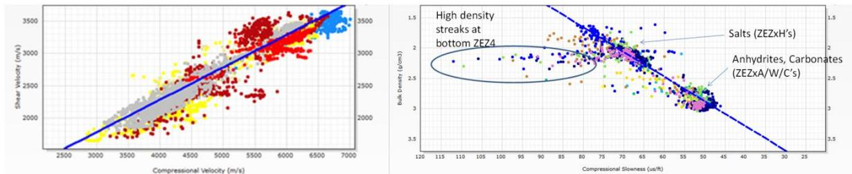
Figure 10: Vp-Vs relation (left) and P wave slowness – density relation (right) of the Zechstein section
