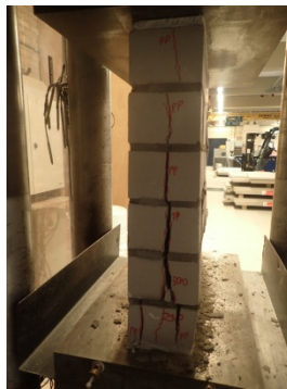
Figure 24 – Crack pattern of specimen TUD_MAT-11Hb tested under vertical compression test (second period).
