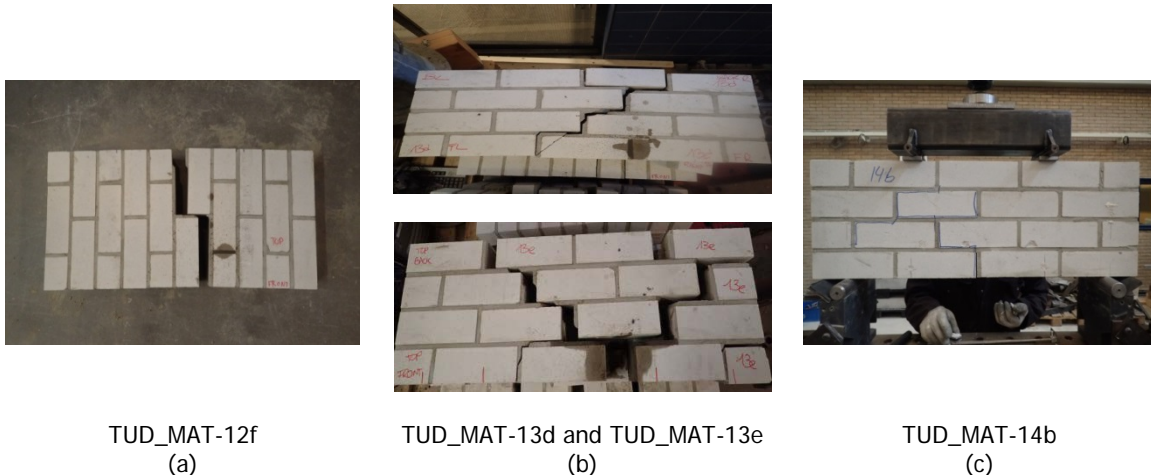
Figure 30 - Crack patterns of calcium silicate masonry specimens subject to: (a) out-of-plane vertical bending test; (b) out-of-plane horizontal bending test; (c) in-plane vertical bending test.
