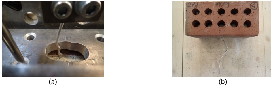
Figure 73 – Crack pattern of specimens TUD_MAT-27: (a) buckling of the tie at the peak force level; (b) final deformed configuration for TUD_MAT-27d.
