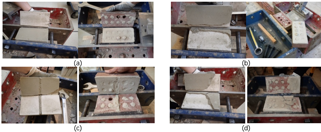
Figure 38 – Observed failure mechanisms: (a) type A in stack bonded specimens; (b) type B and mixed mode type B-C in stack bonded specimens; (c) type B sawn cut specimens; (d) type C in stack bonded specimens.
