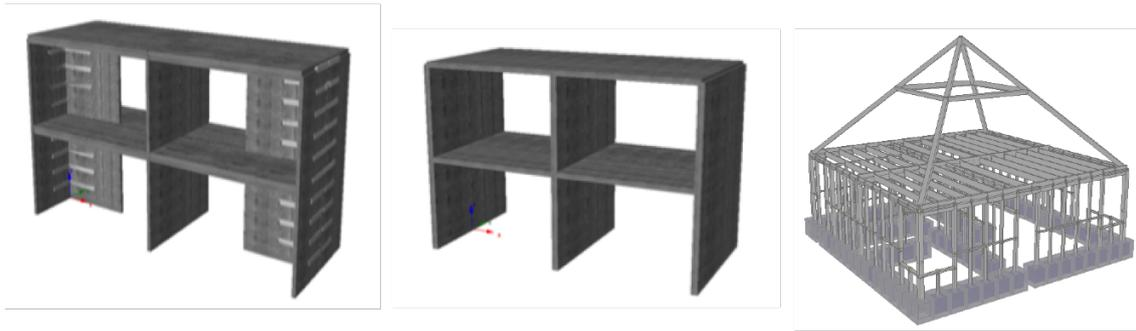
Figure 2.5 Non-URM index building models, left to right: Precast RC wall-slab-wall, Cast-in-place RC wall-slab-wall, Kwelder 8
