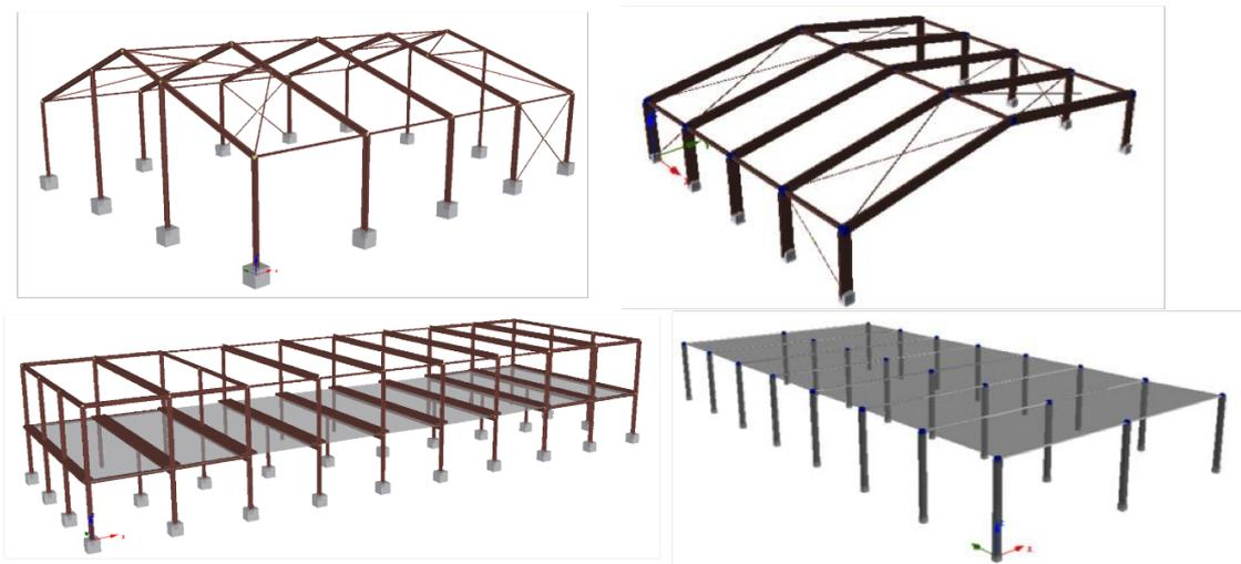
Figure 2.6 Non-URM index building models, clockwise from top left: Beneluxweg 15, Glulam portal frame, RC post and beam (both precast and cast-in-place), Steenweg 19
