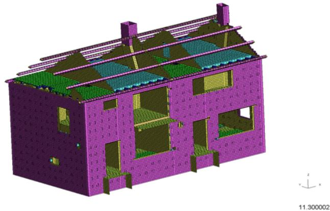
Figure D.6 Collapse state A of LS-DYNA Julianalaan 52 model (Record 8)
