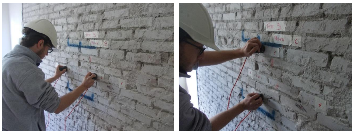
Figure 5. Ultrasonic Test: indirect horizontal configuration (left) and indirect vertical configuration (right).
