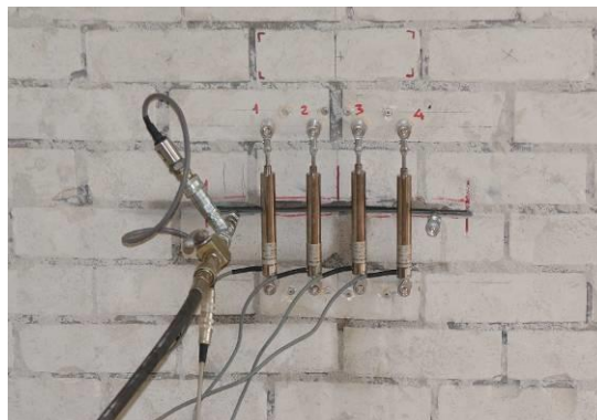
Figure 10. Single Flat Jack Test: increasing of the pressure in the flat jack to restore the slot thickness.
