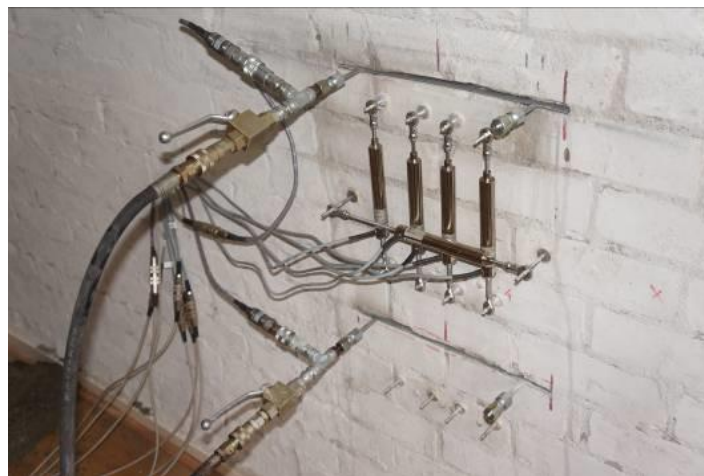
Figure 12 - Double Flatjack Test Setup
