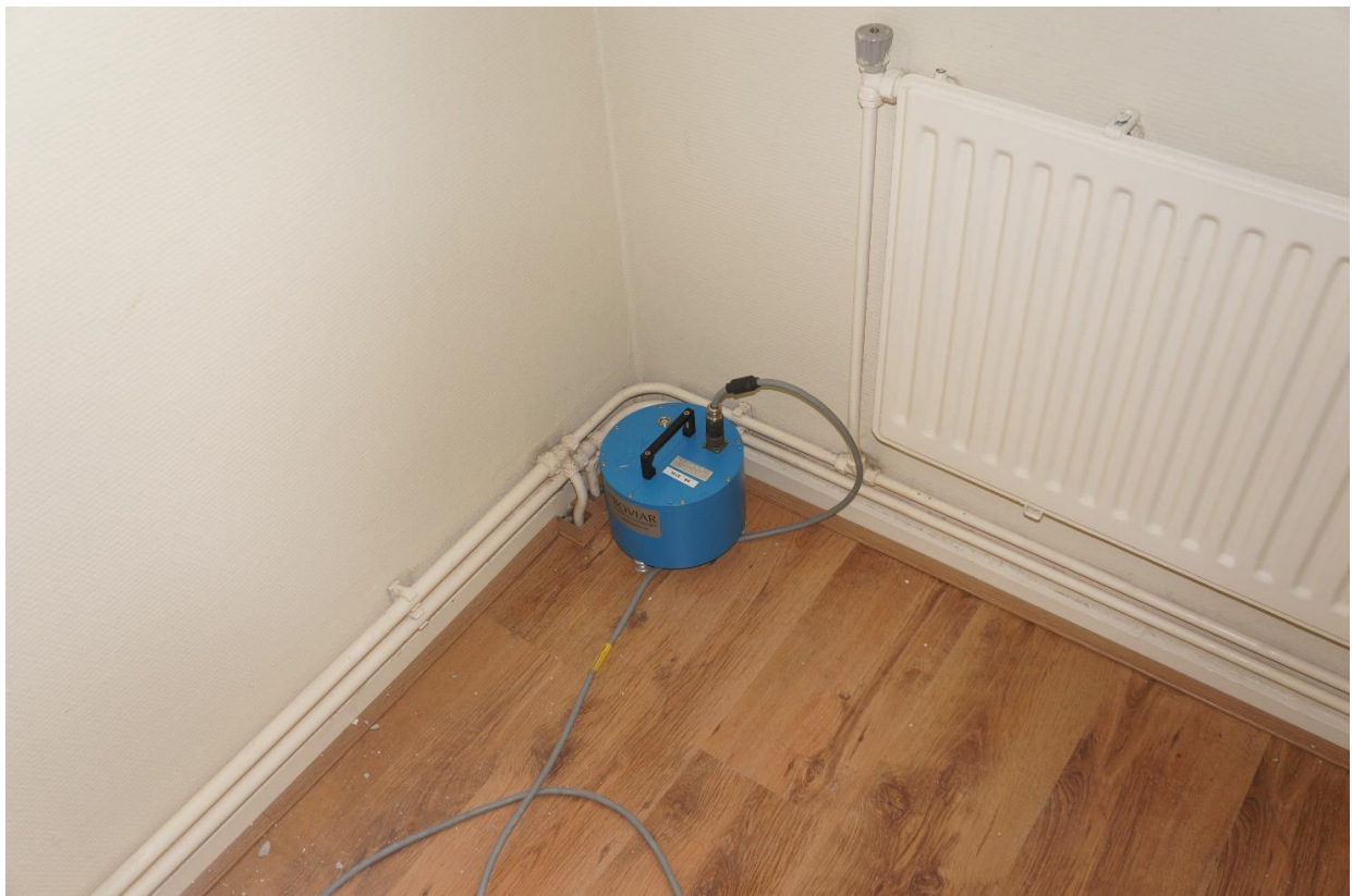
Figure 55. Geophone #7, 2 nd floor, configuration 2
