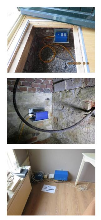
Figure VI.2 Sensors installed on the walls at: crawl space level (top), basement level (middle) and ground floor level (bottom). The large blue box of the lowermost figure is the recorder.
