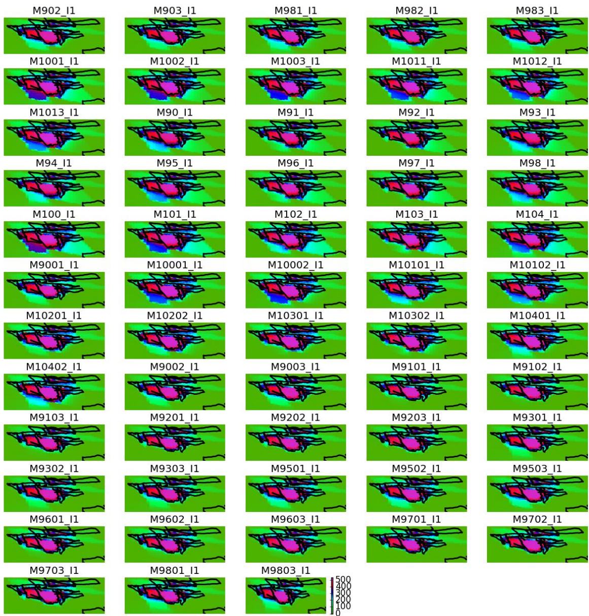
Figure 42. Depletion of the reservoir and adjacent aquifers for the year 2016 for all 58 reservoir scenarios.
