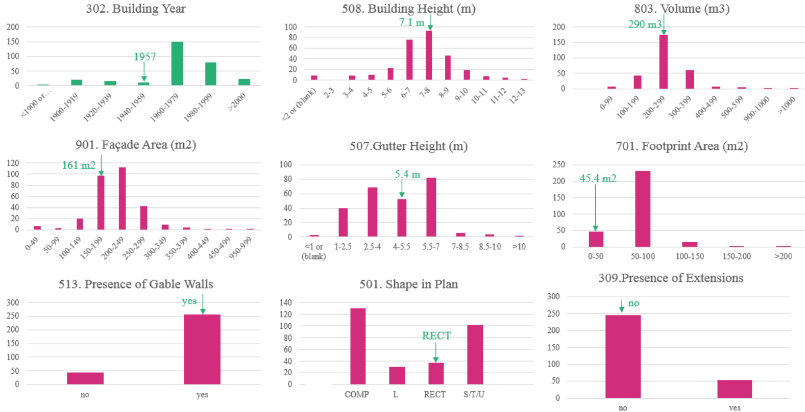
Figure 15 Comparison of the Koningin Julianalaan 52 building's characteristic values to the histograms of the REST300 sample. Vertical axis represents the building count within the sample.
