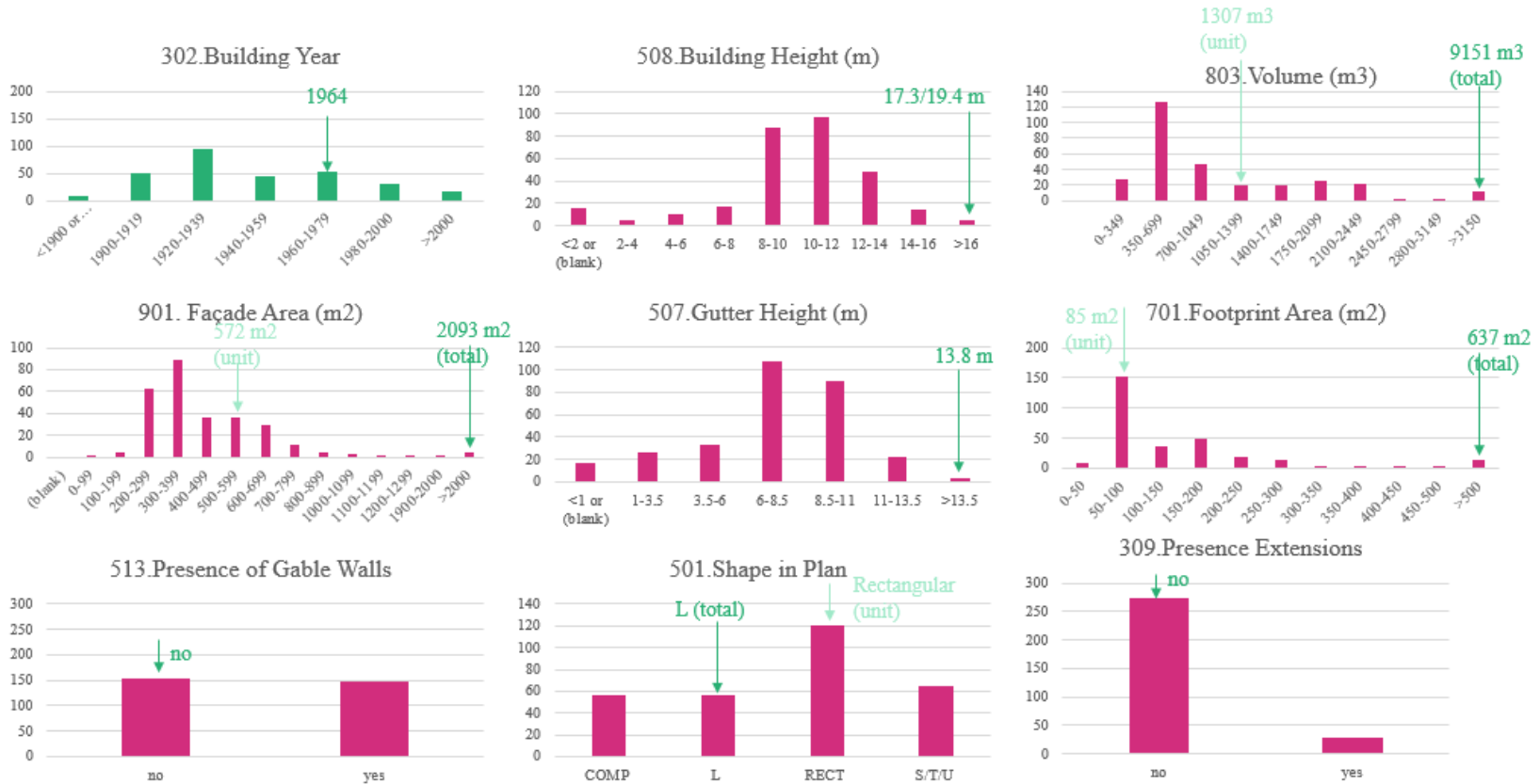
Figure 17 Comparison of the Schuitenzand flat's characteristic values to the histograms of the RESA300 sample. Vertical axis represents the building count within the sample.
