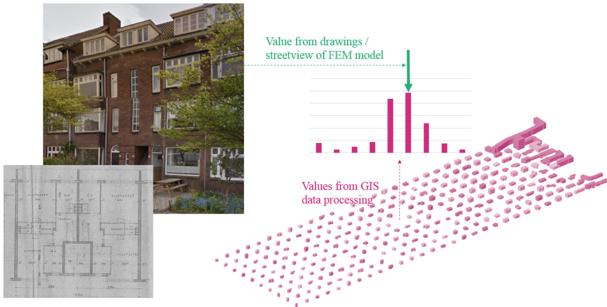
Figure 3 Schematic representation of the different calculation sources for the sample characteristic and distribution and the calculated numerical model characteristic values.
