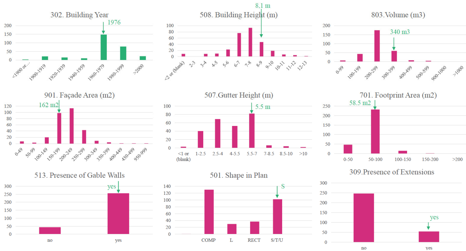
Figure 12 Comparison of the Zijlvest 25 building's characteristic values to the histograms of the REST300 sample. Vertical axis represents the building count within the sample.
