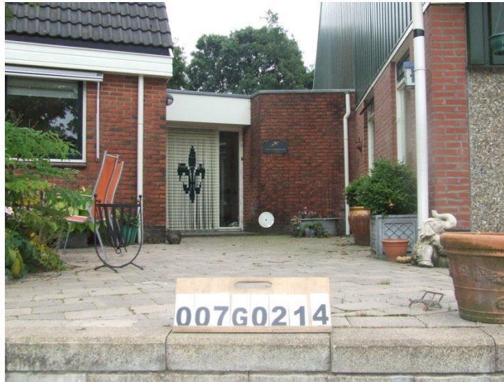
Figure 7b Levelling benchmark 007G0214 approx. 1.3km north-east of 007G0139 shows a constant deformation over time. Linear velocity \sim 5\text{mm/yr} . (values relative to reference benchmark (m))
