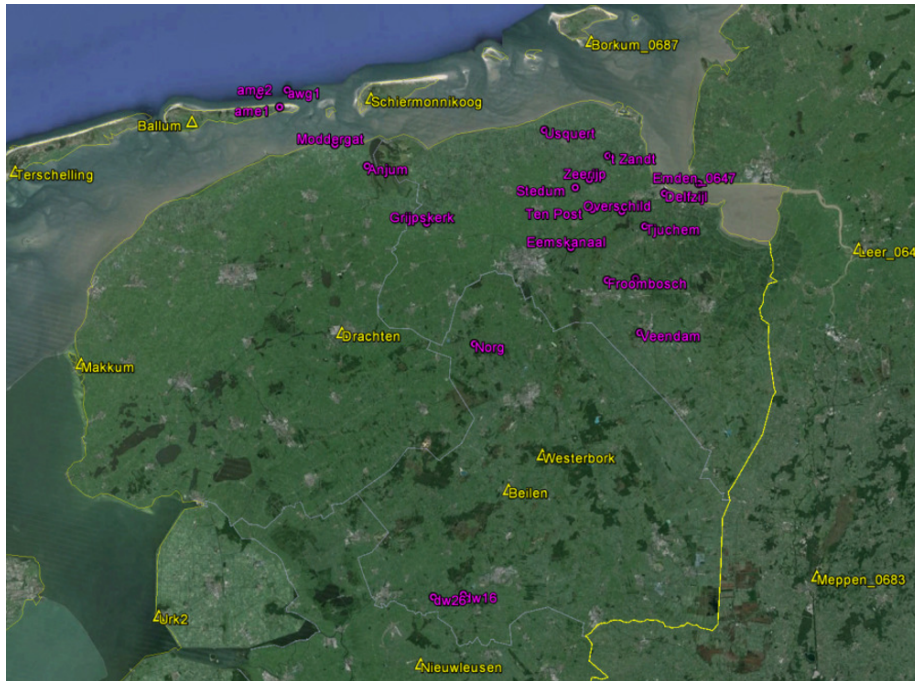
Figure 8: Network of GPS reference and continuous monitor stations (From [19]). The GPS reference stations are the green triangles, the GPS monitor stations are the purple circles. The AGRS.NL station AMEL in Nes Ameland is missing in this figure.
