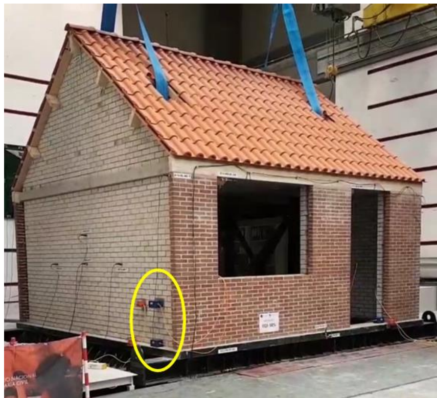
Figure 7.6. Reproduction of the TNO installation of accelerographs at ground level and at a higher level on a full-scale model subjected to shake table testing at LNEC
