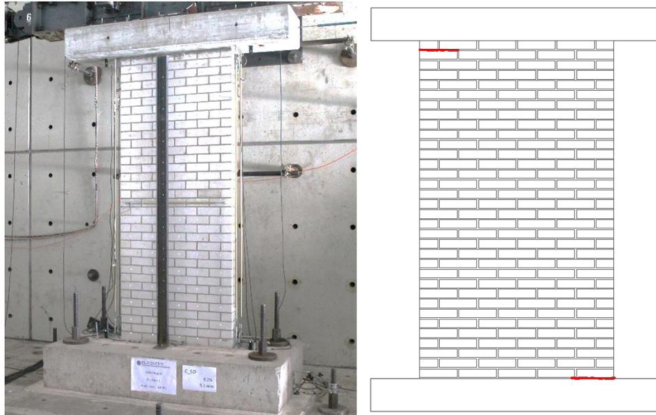
Figure 123. EC\_COMP\_1: crack pattern after CYCLE 5\_D (drift 0.2%).
