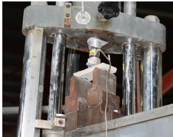
*Figure 7. Bending Test on the mortar specimens taken "in-situ".*
