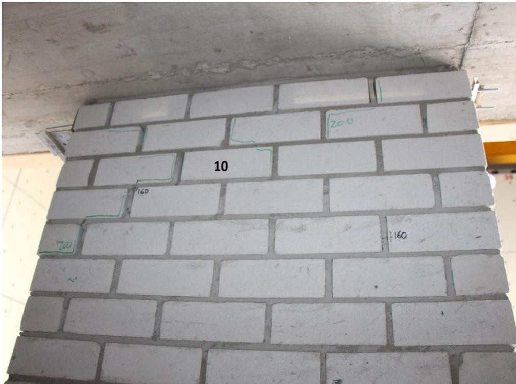
Figure 321. Crack #10 after the test # 23, 200%\_EQ2\_320, PGA= 3.1 m/s<sup>2</sup>
