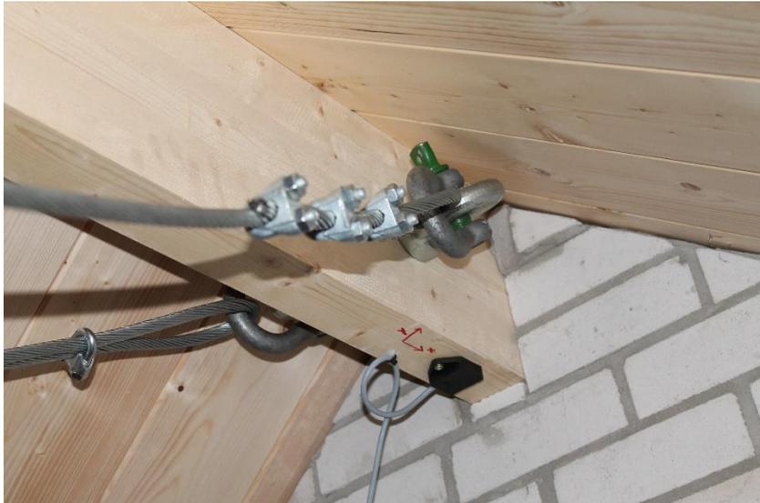
The following picture shows a view of accelerometer #6.
