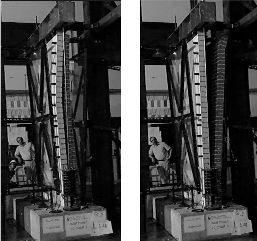
*Figure 230. Deformed shape of the EC\_COMP\_6 Specimen (left and right).*
