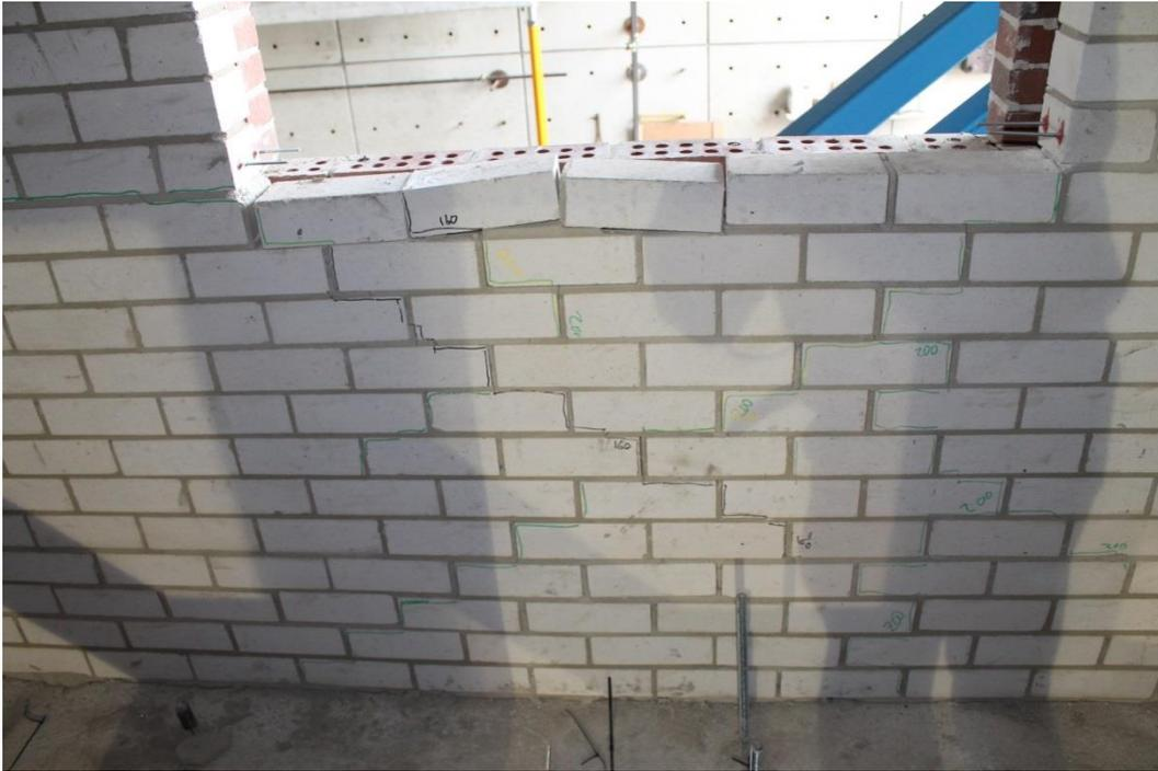
Figure 330. De-cohesion of masonry blocks observed in the calcium silicate masonry, after the test # 23, 200%\_EQ2\_320,  $PGA = 3.1 \text{ m/s}^2$ .
