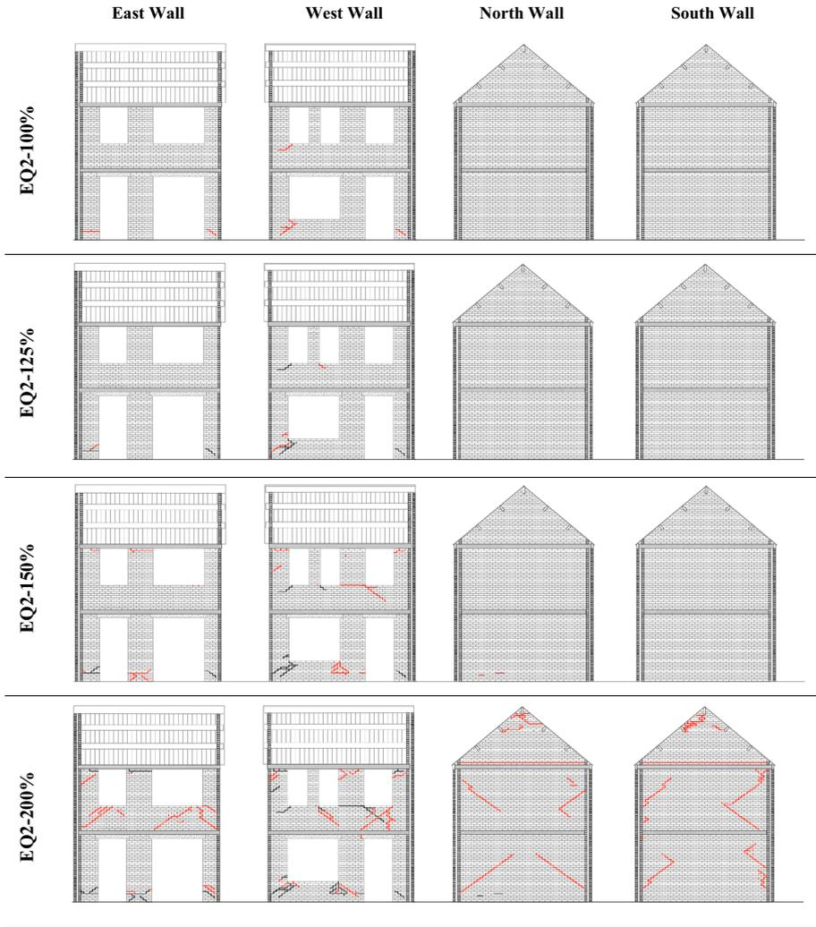
**Fig. 11** Crack pattern evolution of the inner CS walls
