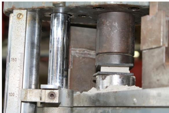
*Figure 8. Compressive Test on half specimen of the mortar taken "in-situ".*
