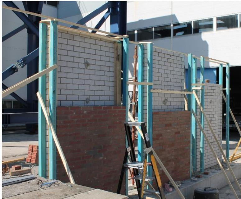
*Figure 166. Cavity Wall Specimens during construction phases.*
