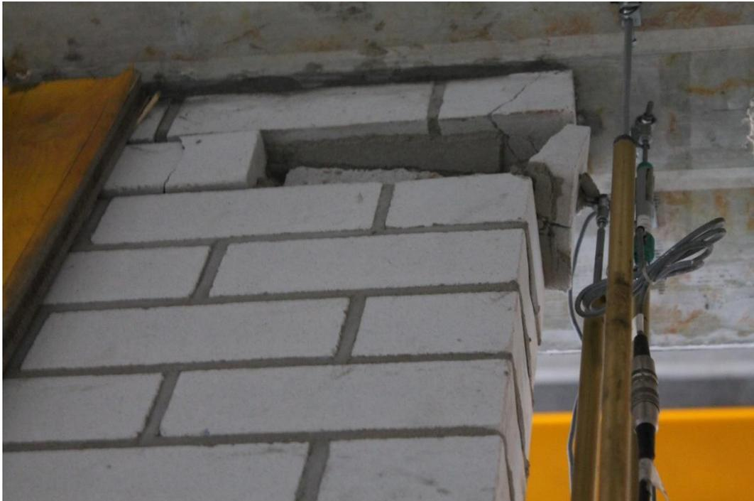
*Figure 131. Expulsion of a portion of masonry due to toe crushing mechanism at the top of the wall, after CYCLE 17\_D (drift 2%).*
