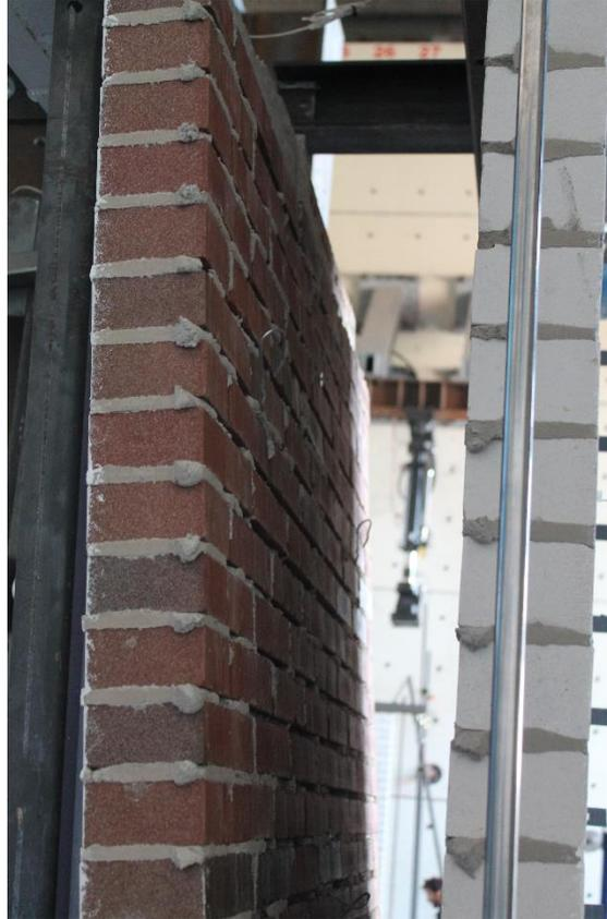
*Figure 232. Separation of the two leaves (during Test 5.1.).*
