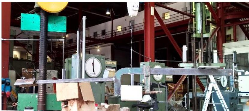
Figure 81. Balanced upper clamp for bond wrench test.
