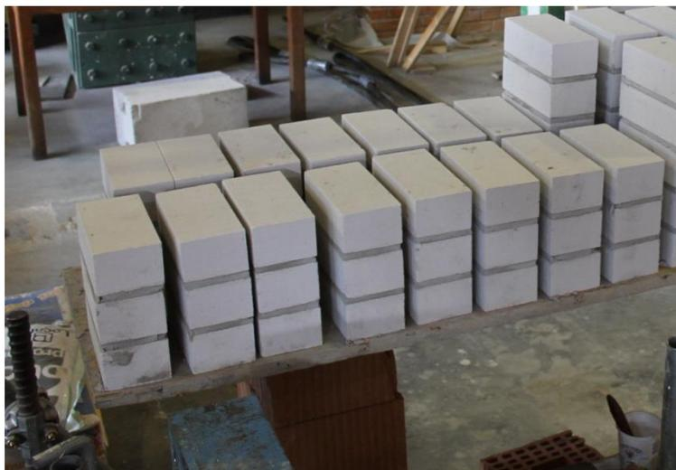
Figure 94. View of the specimens (EC\_MAT\_H\_16\_A/P) for Triplet Test.
