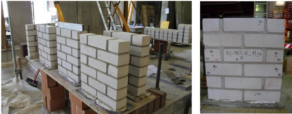
Figure 53. View of the Calcium Silicate Masonry “house” wallets.
