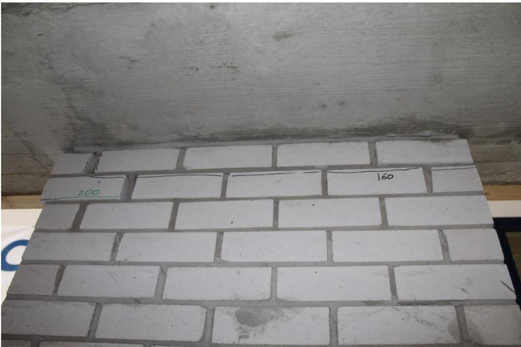
*Figure 327. Horizontal crack due to sliding identified on the top of calcium silicate pier, after the test # 23, 200%\_EQ2\_320,  $PGA = 3.1 \text{ m/s}^2$ .*
