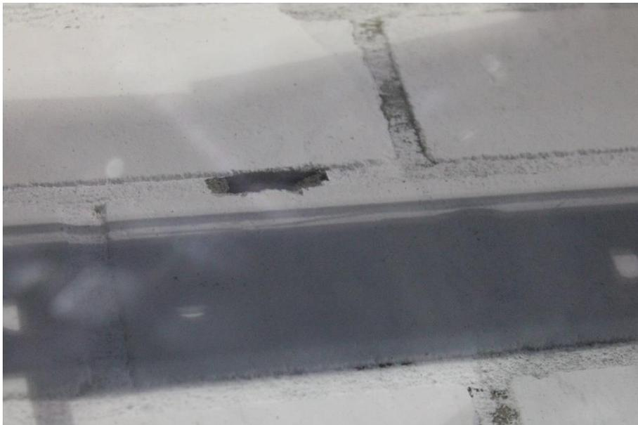
Figure 229. Damage on the Mortar Bed-joint (after Test 5.1.)
