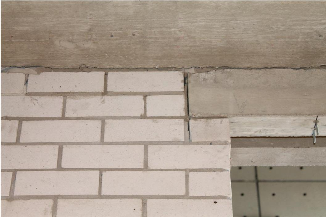
*Figure 326. Sliding of the concrete lintel with respect to the masonry support, after the test # 23, 200%\_EQ2\_320,  $PGA = 3.1 \text{ m/s}^2$ .*
