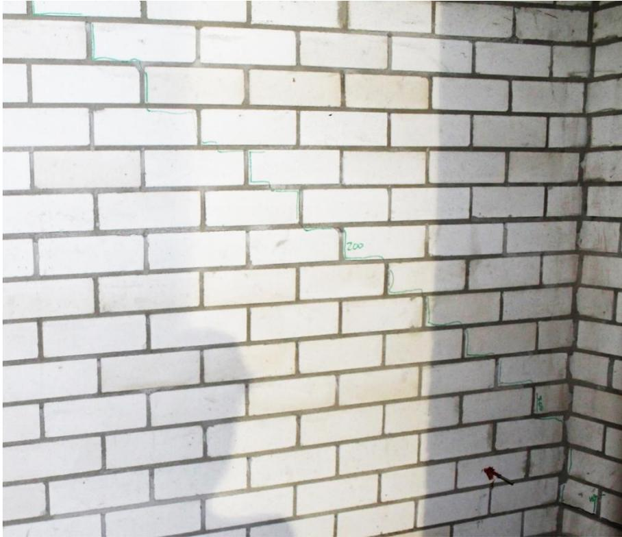
*Figure 324. Crack after the test # 23, 200%\_EQ2\_320,  $PGA= 3.1 \text{ m/s}^2$ .*
