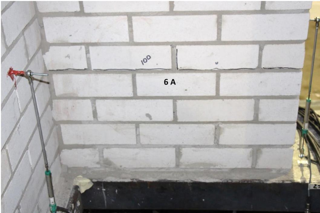
*Figure 308. Crack n 6A after the test # 16, 100%\_EQ2\_160, PGA= 1.6 m/s<sup>2</sup>.*
