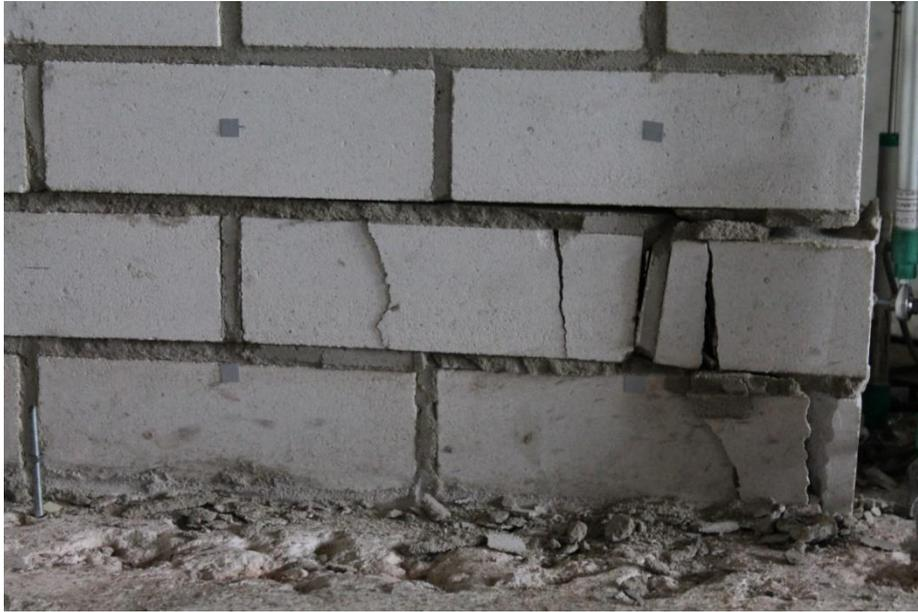
*Figure 128. EC\_COMP\_1. Toe crushing mechanism at the base of the wall, after CYCLE 17\_D (drift 2%).*
