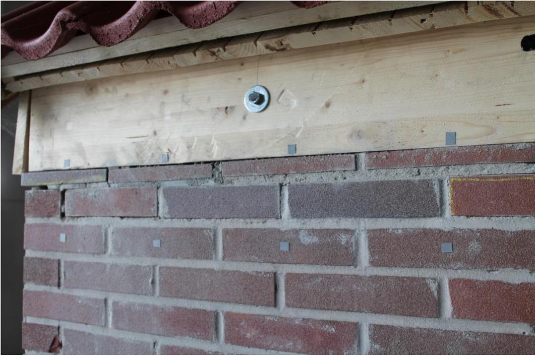
*Figure 334. Crack after the test # 23, 200%\_EQ2\_320, PGA= 3.1 m/s<sup>2</sup>.*
