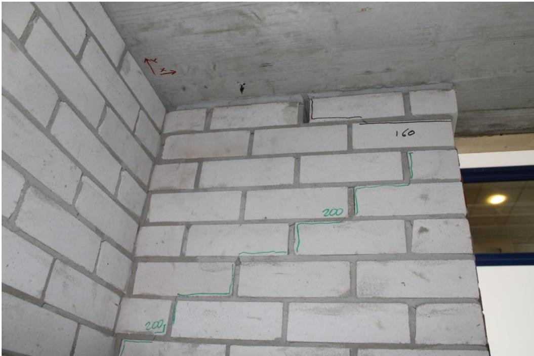
Figure 328 Increase of the sliding observed on the top of the pier and formation of a new stair-stepped crack, after the test # 23, 200%\_EQ2\_320,  $PGA = 3.1 \text{ m/s}^2$ .
