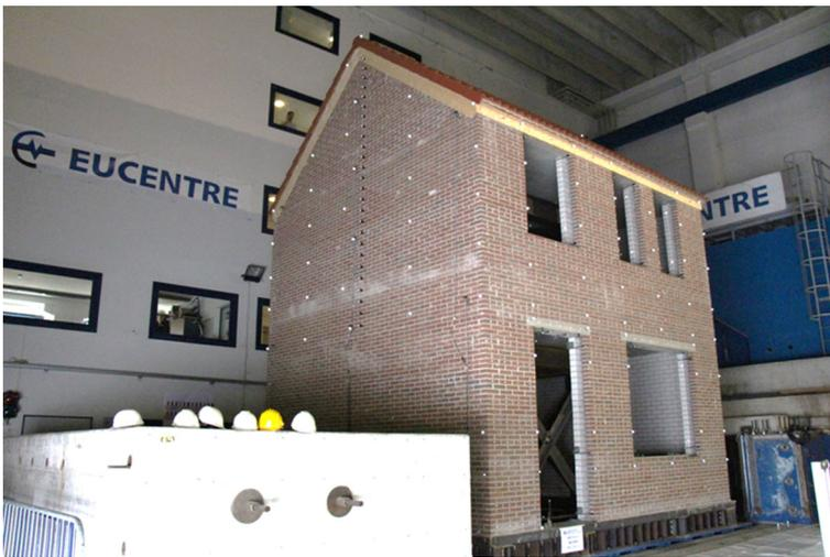
**Fig. 21** 3D optical acquisition system (markers illustrated with *white dots*)
