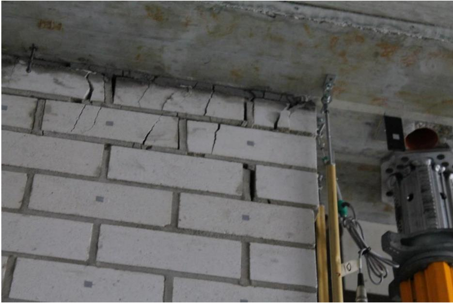
*Figure 130. Toe crushing mechanism at the top of the wall, after CYCLE 17\_D (drift 2%).*
