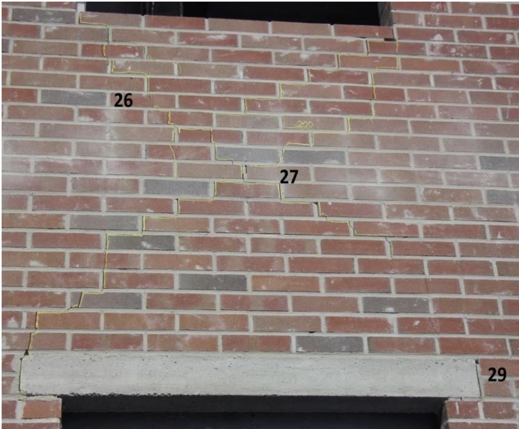
Figure 336. Cracks 26, 27 and 29 after the test #23, 200%\_EQ2\_320, PGA= 3.1 m/s<sup>2</sup>.
