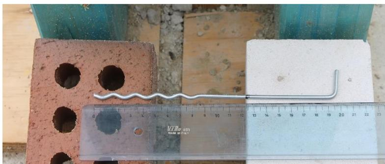
*Figure 278. Ties dimensions and geometry.*
