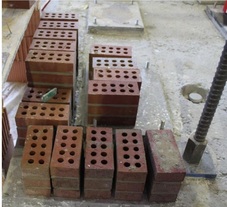
Figure 97. View of part of the specimens (EC\_MAT\_H\_26\_A/P) for Triplet Test.
