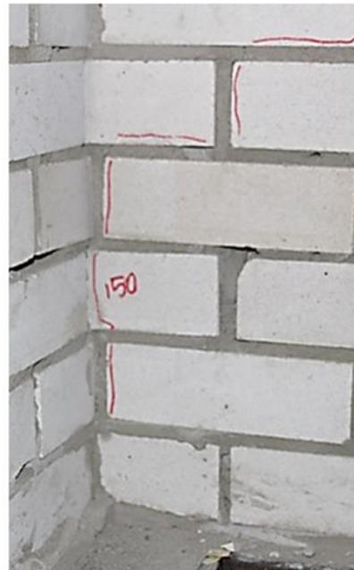
Figure 312. Cracks #14 and #14B after the test # 19, 125%\_EQ2\_200, PGA=  $2 \text{ m/s}^2$ .
