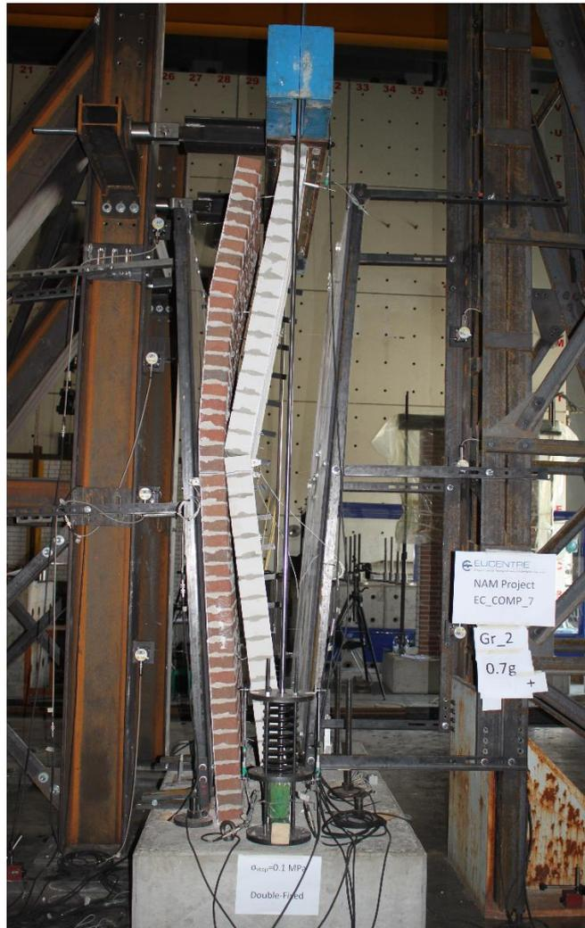
*Figure 252. Collapse of EC\_COMP\_7 Specimen.*
