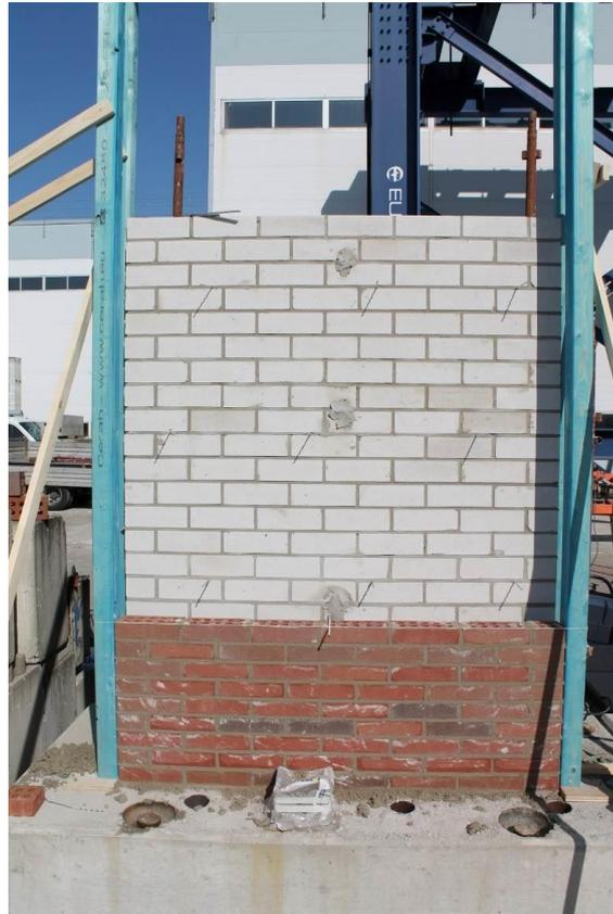
*Figure 165. EC\_COMP\_7 Specimen during construction phases.*
