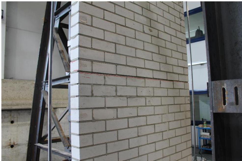
*Figure 196. View of the Mid-height Crack.*
