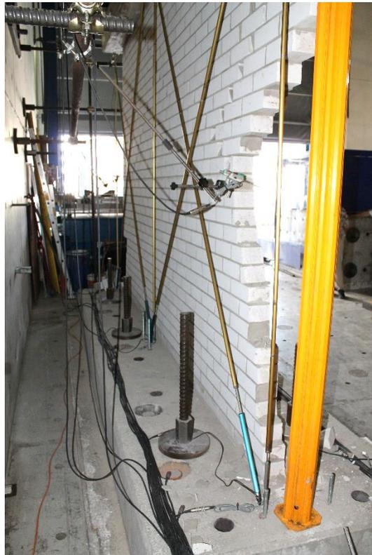
Figure 146 EC\_COMP\_3. Back view of the partial collapse of the wall after CYCLE C\_7D (drift 0.3%).
