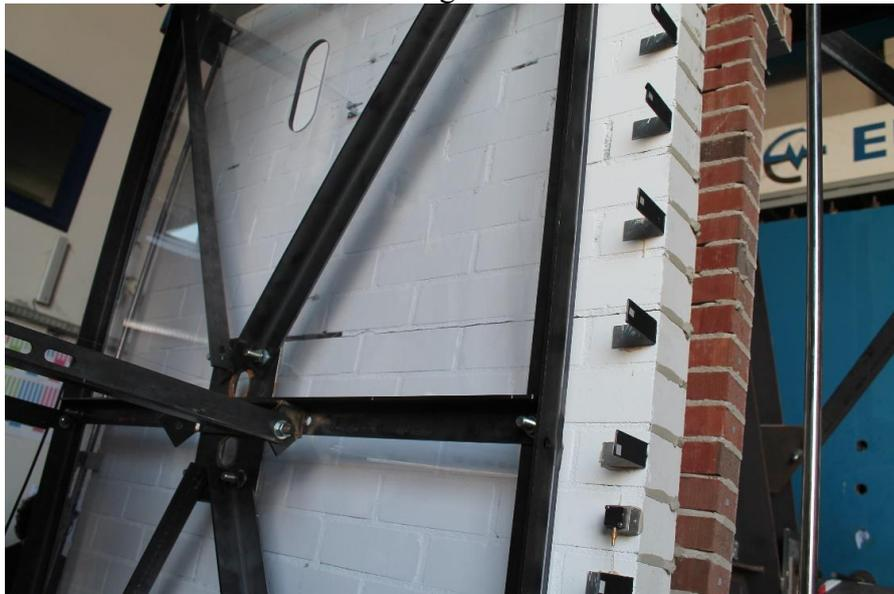
*Figure 231. Formation of mid-height crack (after Test 5.1.).*
