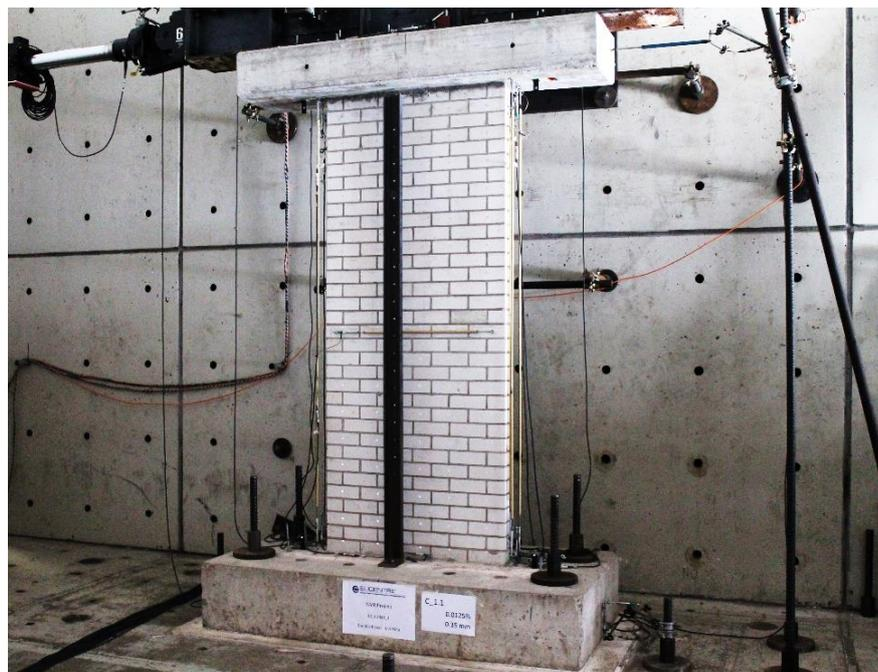
*Figure 122. EC\_COMP\_1: Test set-up.*
