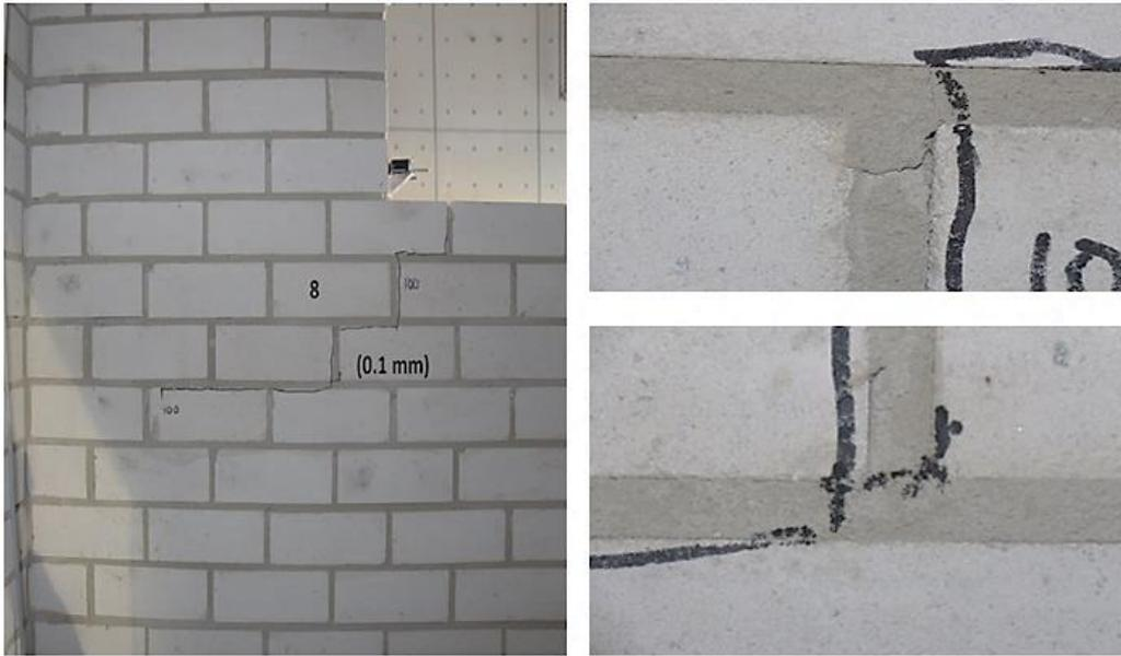
Figure 310. Crack #8 after the test # 16, EQ2\_160%, PGA= 1.6 m/s<sup>2</sup>
