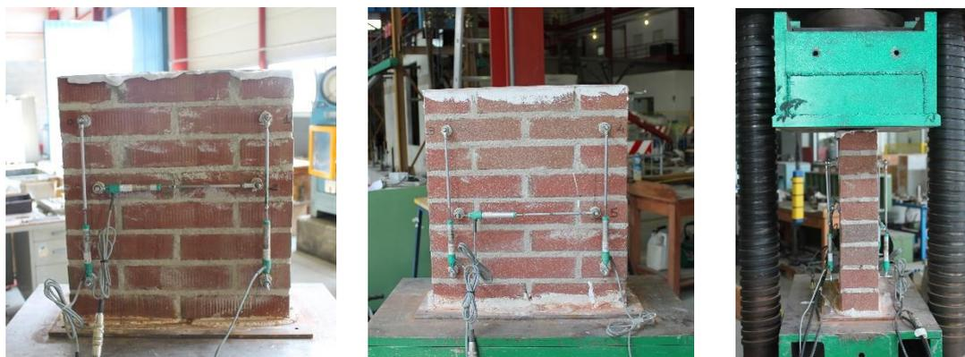
*Figure 41. Setup of the compressive test on clay masonry wallettes*
