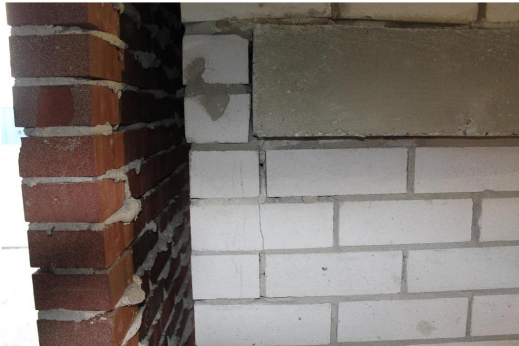
Figure 329. Fracture of brick at the interface between flange and S wall, after the test # 23, 200%\_EQ2\_320,  $PGA = 3.2 \text{ m/s}^2$ .
