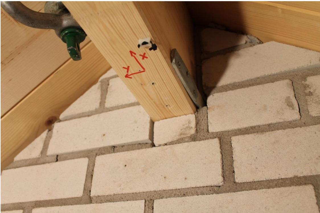
Figure 331. Cracks around the timber beams due to pounding of the beams on the supporting masonry gable walls, after the test # 23, 200%\_EQ2\_320,  $PGA = 3.1 \text{ m/s}^2$ .
