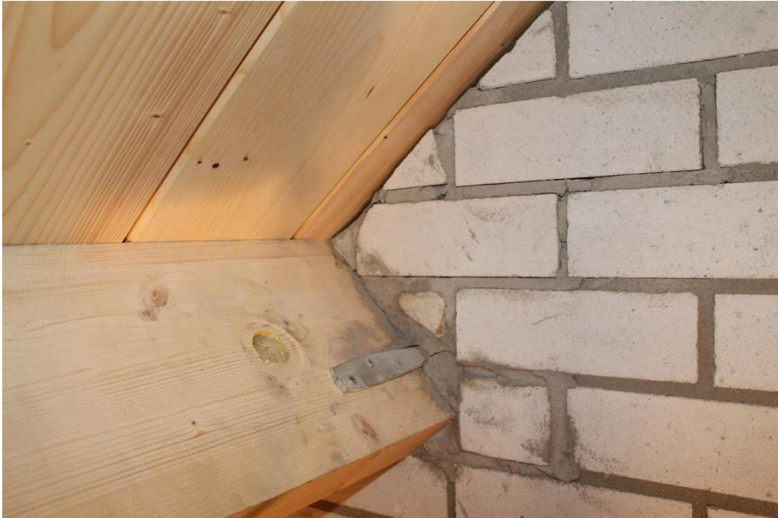
*Figure 332. Cracks around the timber beams due to pounding of the beams on the supporting masonry gable walls, after the test # 23, 200%\_EQ2\_320,  $PGA= 3.1 \text{ m/s}^2$ .*
