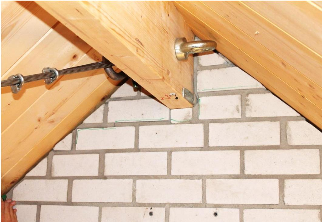
*Figure 346. Cracks observed around the ridge timber beam due to pounding (after the test #29, 60%\_EQ2\_100, PGA= 1.0 m/s<sup>2</sup>).*
