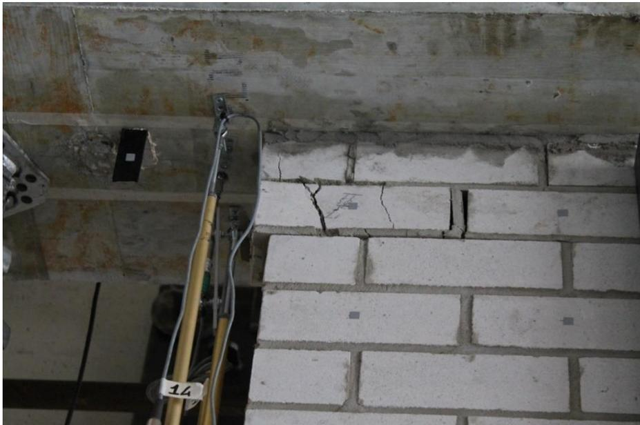
*Figure 129. EC\_COMP\_1. Toe crushing mechanism at the top of the wall (actuator side), after CYCLE 17\_D (drift 2%).*
