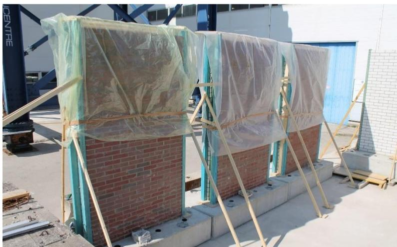
*Figure 169. Cavity Wall Specimens (Clay side).*
