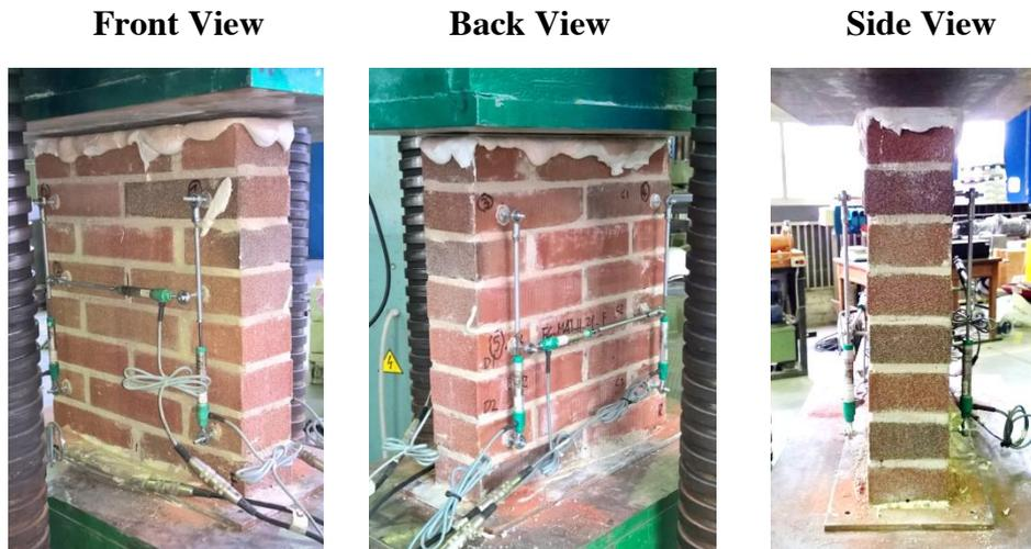
Figure 68. Setup of the compressive test on clay masonry wallettes.
