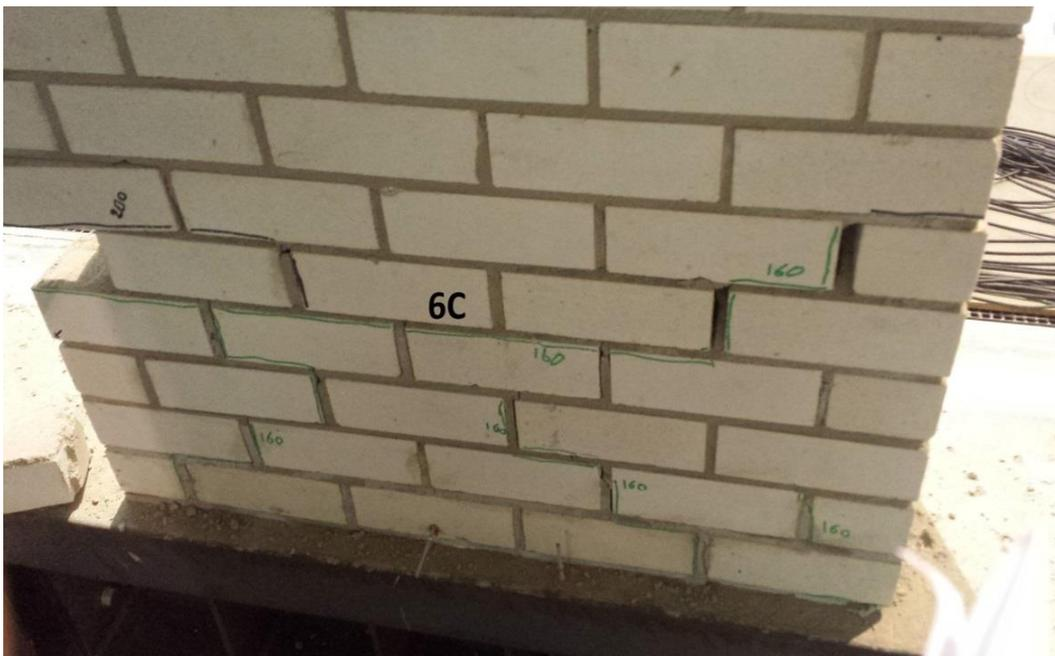
*Figure 315. Crack #6C after the test # 21, 150%\_EQ2\_240, PGA=  $2.4 \text{ m/s}^2$ .*
