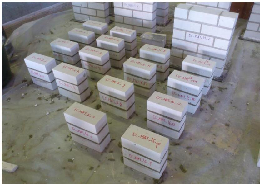
Figure 92. View of the specimens (EC\_MAT\_16\_a/p) for Triplet Test.
