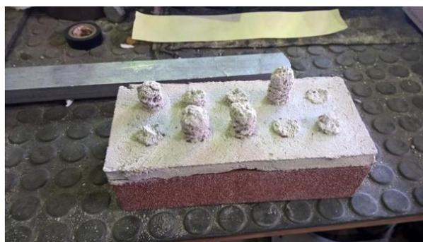
Figure 86. Test performed on clay specimens - failure of the joint.
