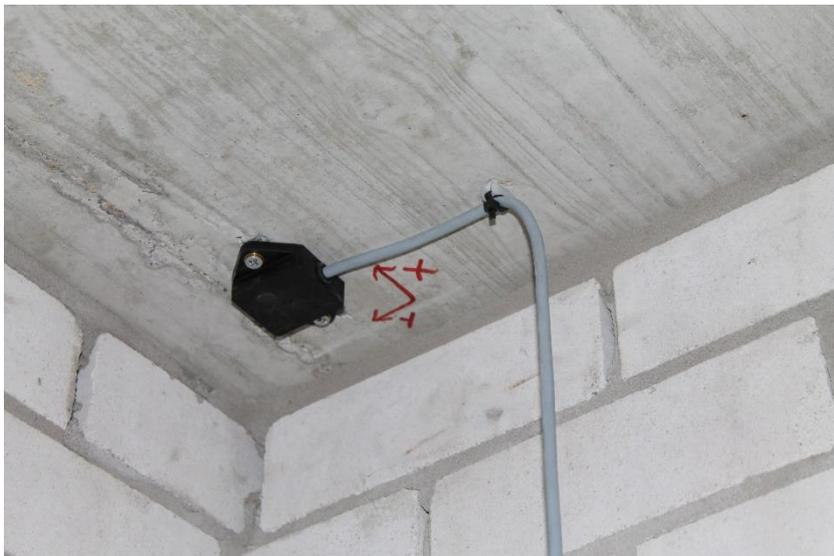
The following picture shows a view of the accelerometer #25 and the wire of the potentiometer #9.
