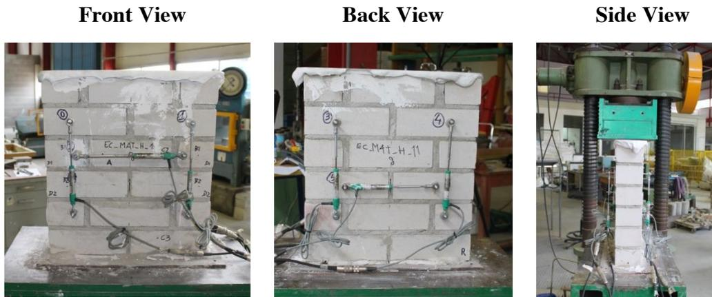
Figure 55. Setup of the compressive test on CS masonry wallettes.
