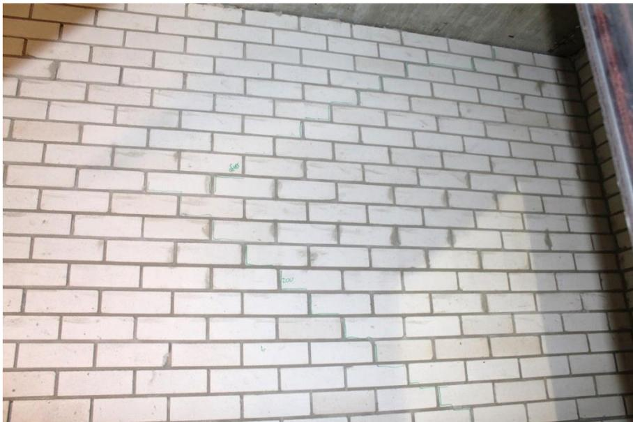
*Figure 325. Crack after the test # 23, 200%\_EQ2\_320,  $PGA= 3.1 \text{ m/s}^2$ .*
