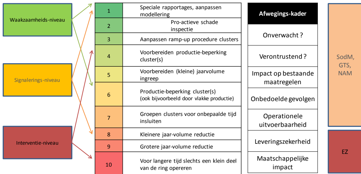
Figure 29 Coupling of control measures to the MRP threshold levels. For detailed description see reference 1.
