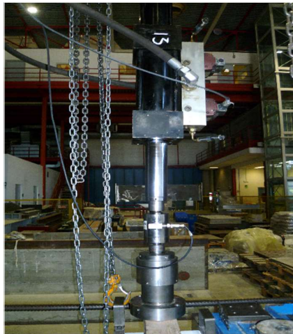
Figure 2:25: Actuator used to apply shear load to the specimen.
