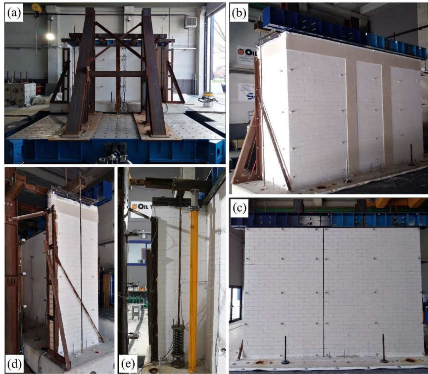
Figure 3:12: Testing layout: general view of the shaking table and the testing setup (a), general view of CS-000-RF2 (plaster applied to investigate non-structural damage, more details in section 3.2.3.2) (b) and CS-000-L1&L2 (c), return wall restrain system fixed with diagonal to the rigid frame (d), spring system for the application of the top overburden pressure and support for the uplift of the top beam (e).
