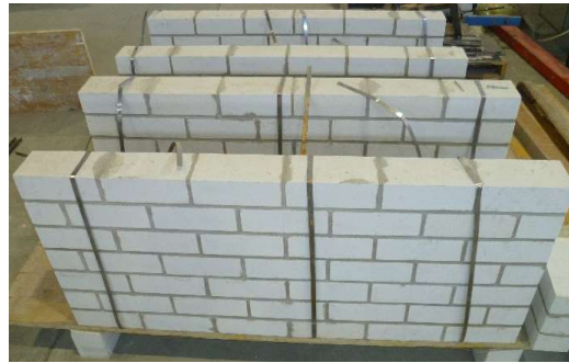
Figure 2:42: CS masonry specimens tested for flexural strength in the laboratory.
