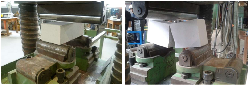
Figure 2:9: Test setup in the laboratory (right) and failure of CS units (left) during determination of flexural strength of units.
