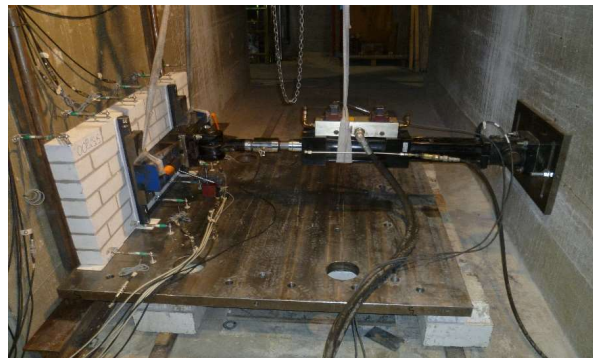
Figure 2:45: Test setup adopted in the laboratory for determining the flexural strength of masonry.
