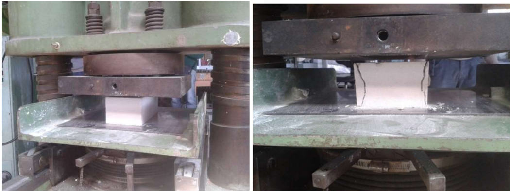
Figure 2:6: Test setup in the laboratory (right) and failure of CS units (left) during determination of compressive strength of units.
