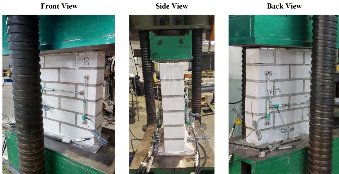
Figure 2:15: An instrumented CS compression wallette in the laboratory.
