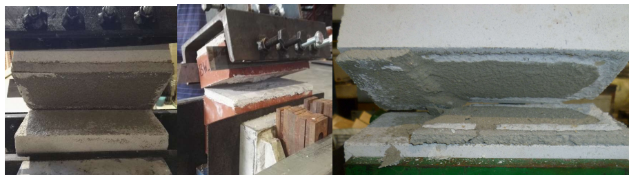
Figure 2:38: Example of failure modes from bond wrench tests in the laboratory.
