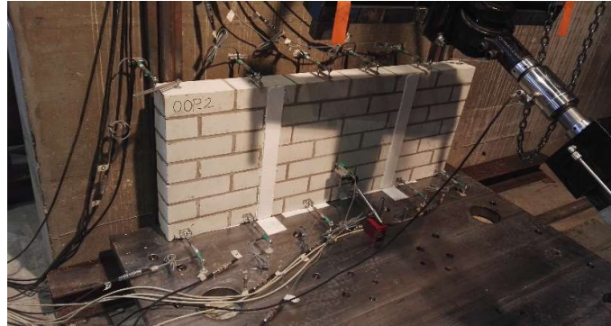
Figure 2:44: Instrumentation used for each specimen.
