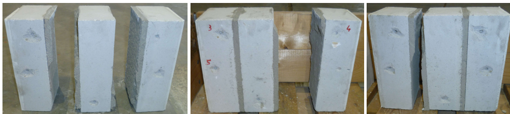
Figure 2:27: Failure modes observed for CS masonry triplets in the laboratory.
