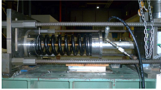
Figure 2:24: Part of test apparatus used to apply vertical pre-compression and accommodate dilatancy.
