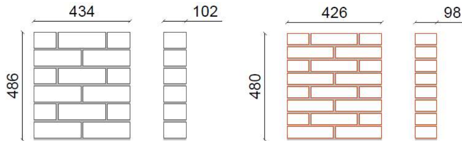
Figure 2:12: Schematic of tested CS (left) and clay (right) masonry compression wallettes.
