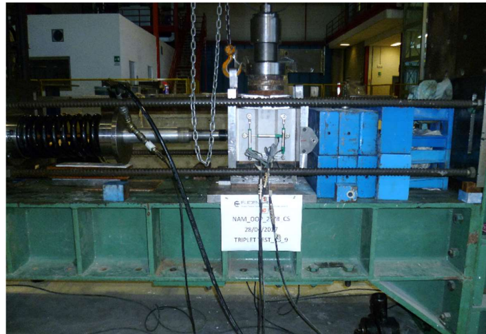
Figure 2:26: Test set-up in laboratory for evaluating the shear strength of masonry joints.
