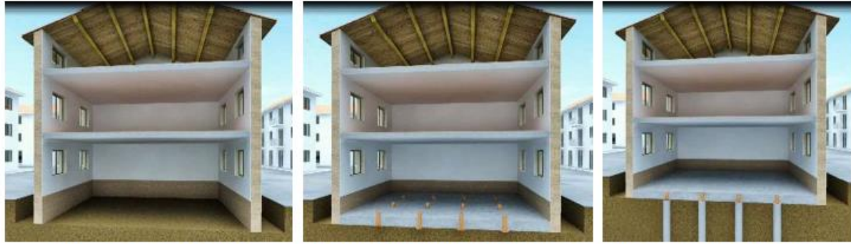
From left to right: Phase 1 "Demolition of ground floor"; Phase 2 "Construction of new foundations: RC slab and piles"
