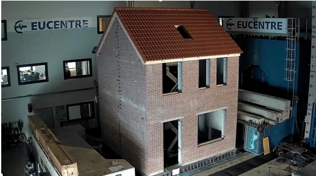
Figure 10.6 Full-scale terraced house unit tested on a shake-table
