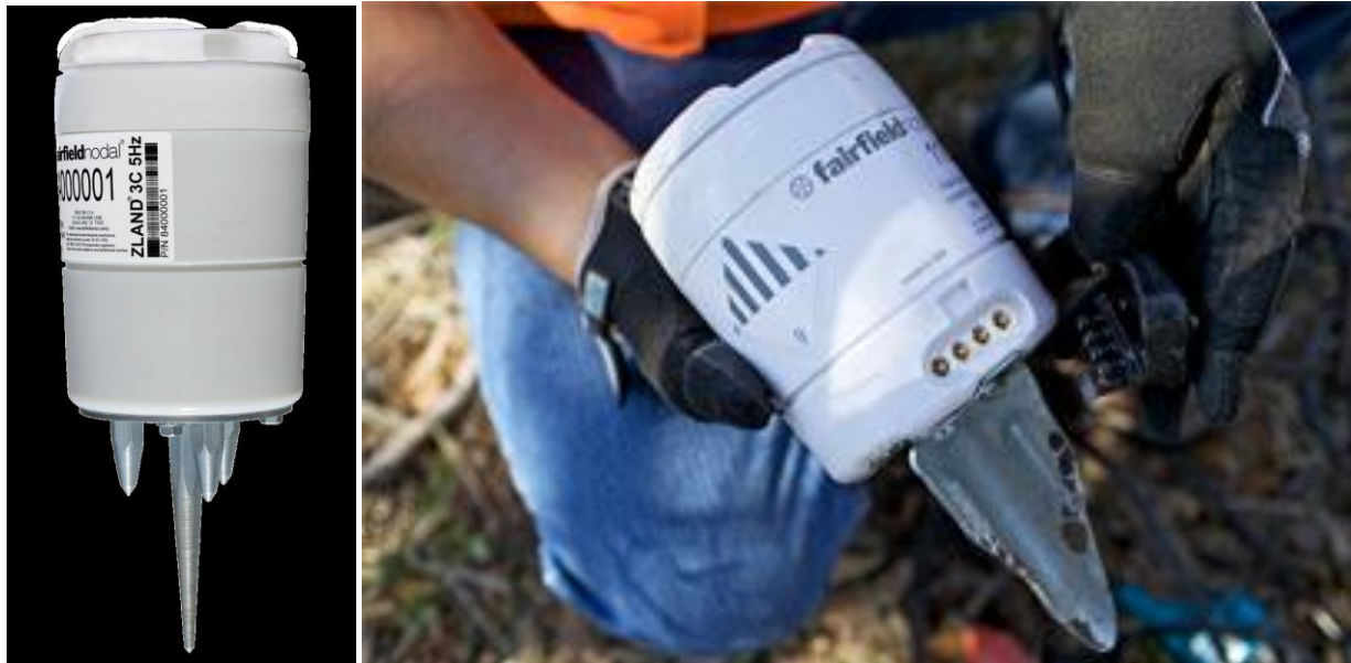
Figure 8.1 Example of a standalone 3C geophones/recorders, so called nodes.
