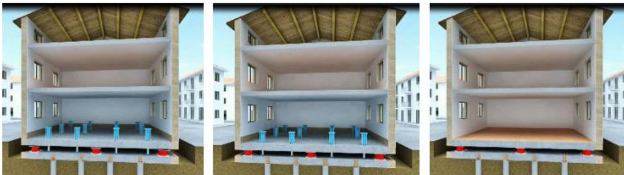
From left to right: Phase 6 "Installation of isolation devices"; Phase 7 "Lowering and finishing works"
