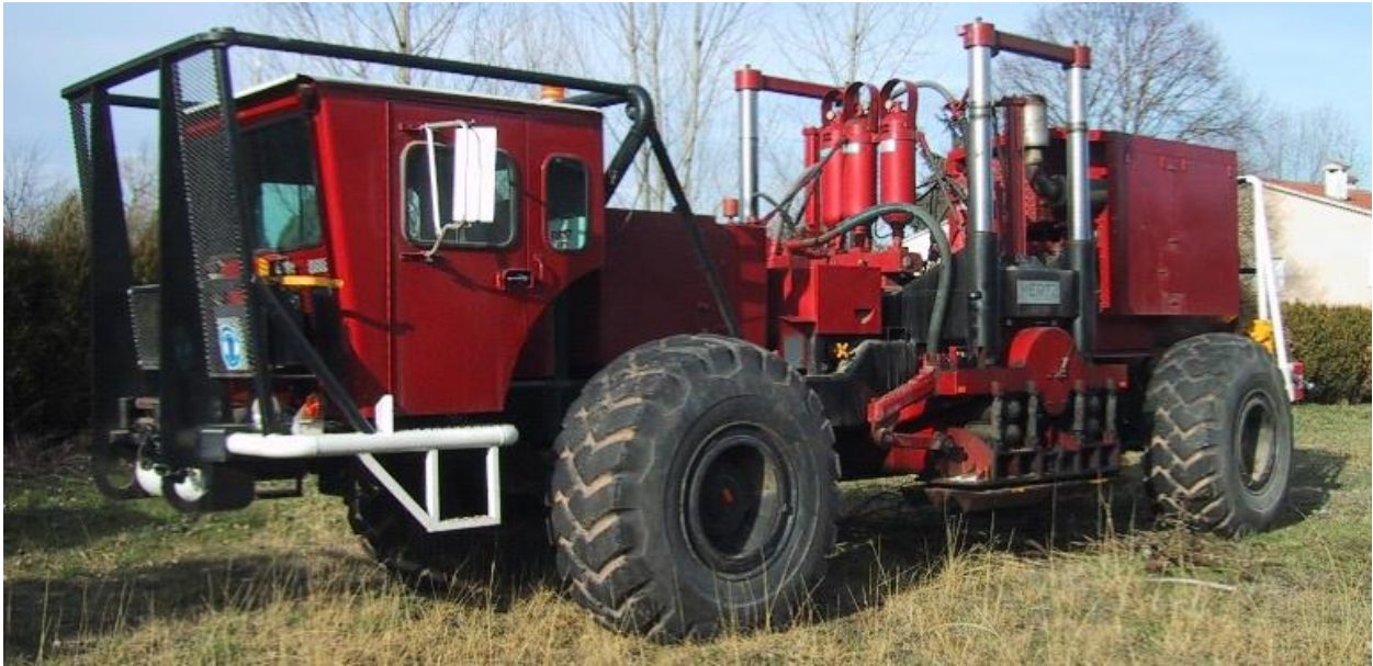
Figure 9.1 One of the last existing S-vibrators in the south of France. Currently investigation whether this vibrator can be restored focus in Groningen are in progress.
