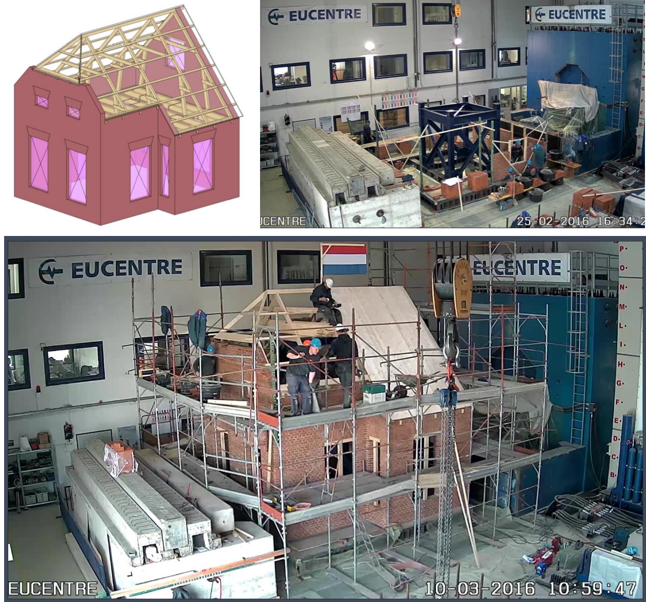
Figure 10.7 Full-scale detached masonry house unit tested on a shake-table
