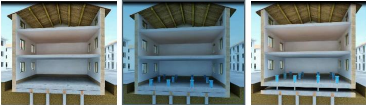
From left to right: Phase 3 "Construction of a new RC upper slab"; Phase 4 "Installation of jacks"; Phase 5 "Uplifting"
