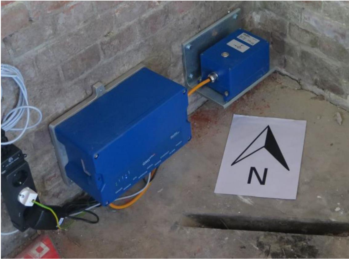
Figure 3.16 Vibration monitoring system – recorder (left) and sensor (right)
