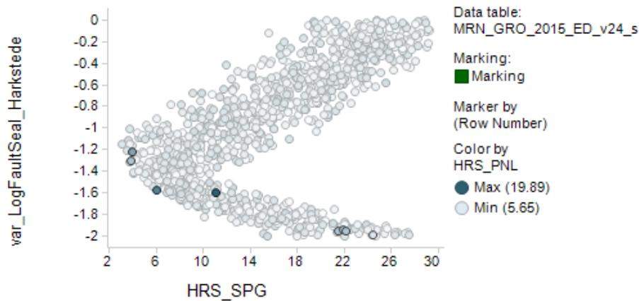
**Figure 62 Example of a local RMSE for the Harkstede mismatch to SPG dependency on a fault sealing factor separating it from the main Groningen field**
