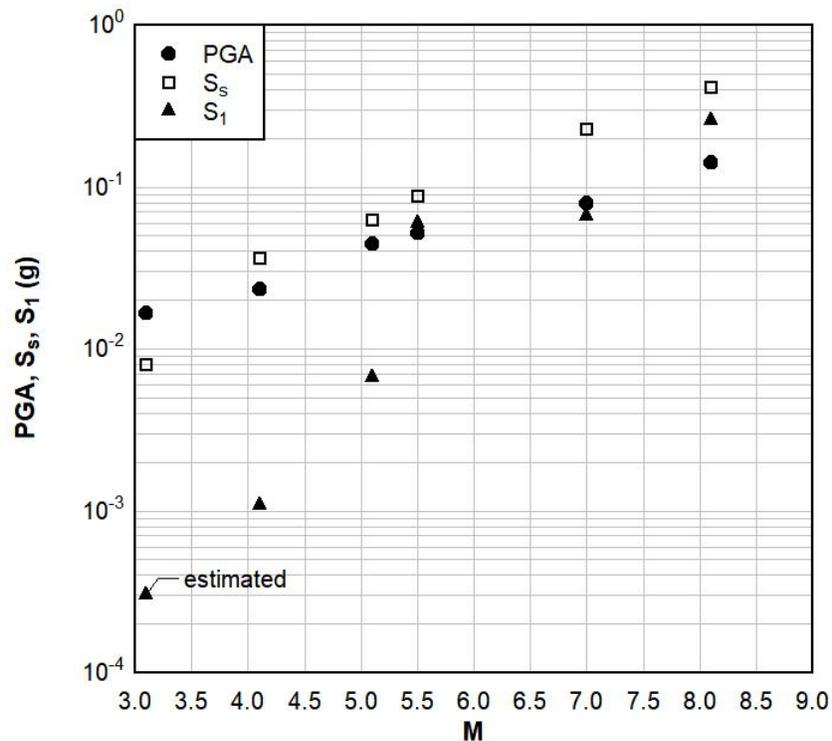
**Figure 1.** Peak ground acceleration and spectral accelerations for 0.2-s and 1.0-s period oscillators vs. earthquake magnitude for motions recorded by the Guerrero accelerograph array in Mexico in 1985 and 1986. All the stations were on hard rock and all the events have epicenters about 25 km from the station.
