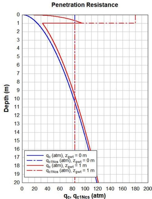
**Figure 6.** Corrected and uncorrected CPT tip resistances ( $q_{c1Ncs}$  and  $q_c$ , respectively) for the very susceptible ( $z_{gwt} = 0$  m) and extremely susceptible ( $z_{gwt} = 1$  m) profiles.
