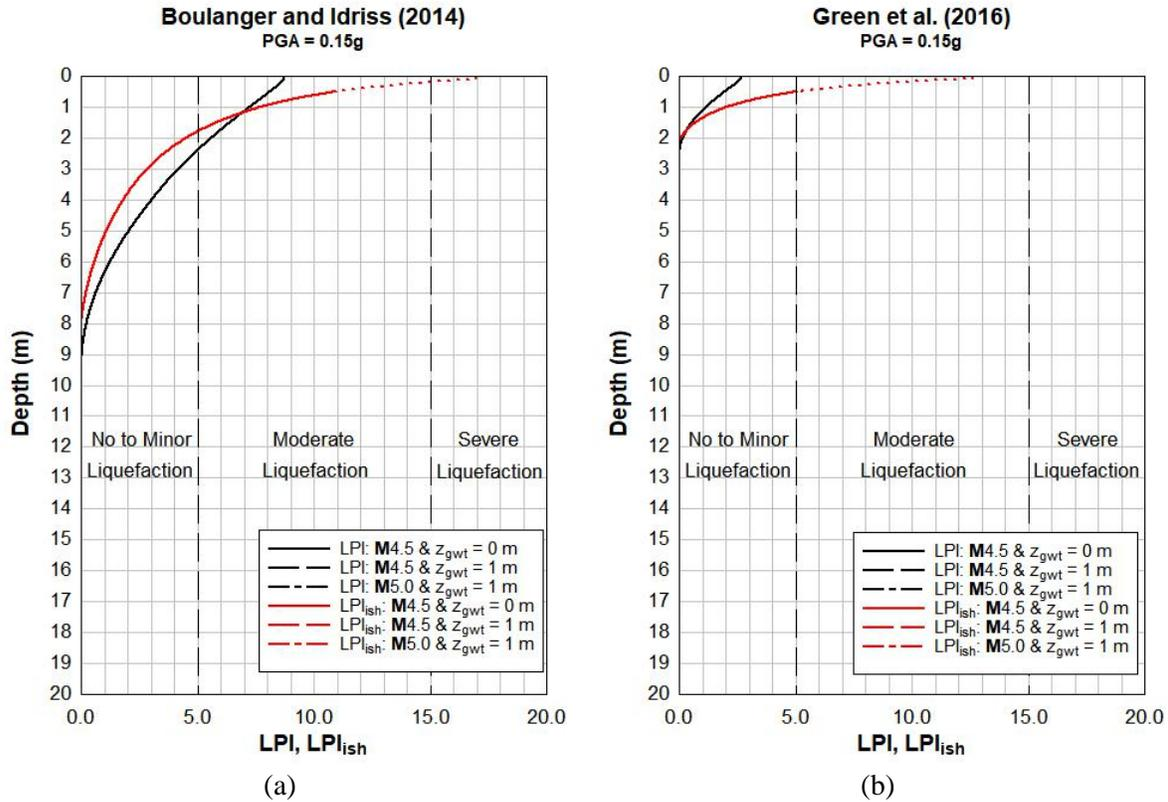
**Figure 5.** Results from the liquefaction parametric study on “very susceptible” (i.e.,  $q_{c1Ncs} = 84$  atm and  $z_{gwt} = 1$  m) and “extremely susceptible” (i.e.,  $q_{c1Ncs} = 84$  atm and  $z_{gwt} = 0$  m) profiles: (a) Computed LPI and  $LPI_{ish}$  profiles using the BI14 CPT-based simplified procedure; and (b) computed LPI and  $LPI_{ish}$  profiles using the Gea16 CPT-based simplified procedure.
