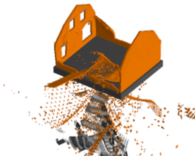
Figure 2.4: Nieuwstraat – Screenshot of collapse mechanism under record N_00451T
