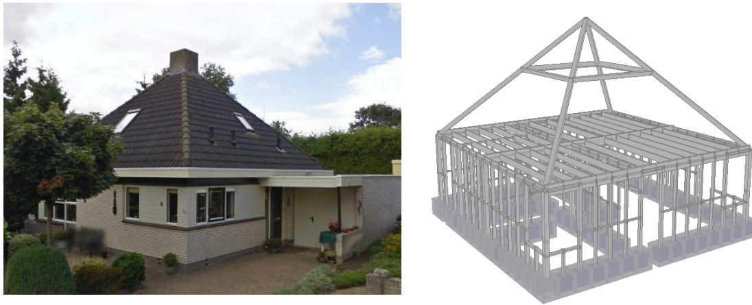
Figure 3.1: Kwelder 8 timber frame/panel house from Google Street View (left) and the corresponding SeismoStruct model (right)
