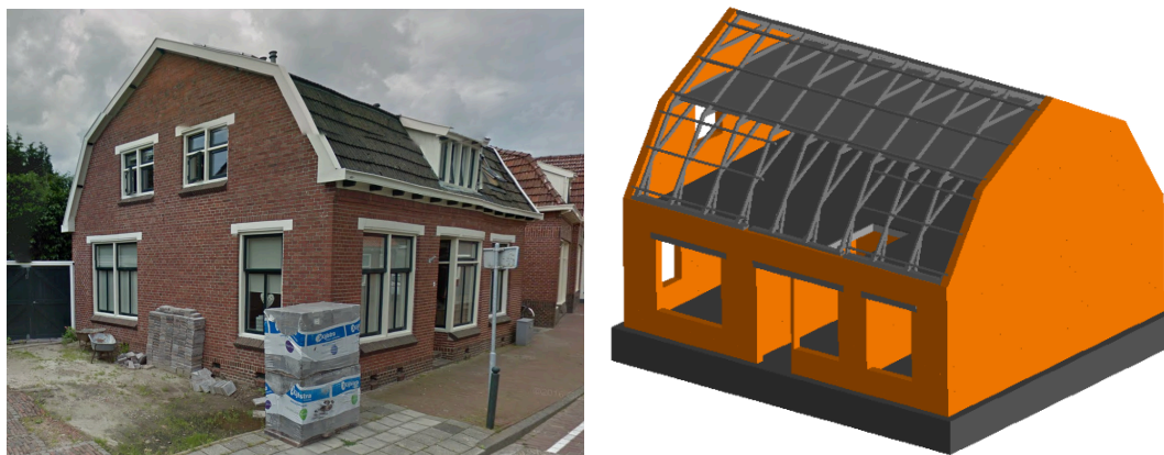
Figure 2.1: Nieuwstraat 8 house from Google Street View (left) and the corresponding ELS model (right) – note that roof tile elements are not shown in the ELS model, so as to allow the visualisation of the roof structure
