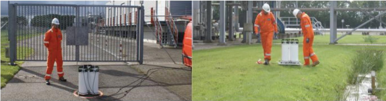
Figure 4: Example of transferred gravity station measured in the past surveys (Leermens, #516). The original gravity station was inside a control room which was demolished after 2001 (right). The new gravity station (left) was established in a close vicinity of the old point. The gravity values between the two points were transferred with dedicated gravity gradient measurements (photo Ref. [5]).
