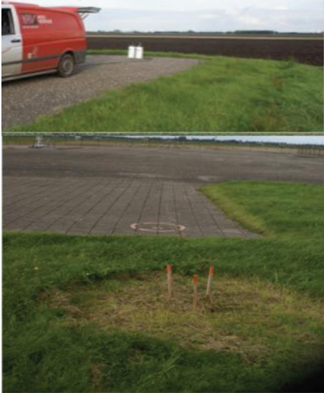
Figure 11: Gravity station Schildmeer (#510). Observation but where gravity was measured was removed after 2001. New gravity station was established on asphalt outside facility fence. The plot on the right shows measured gravity changes. Picture Ref. [5].
