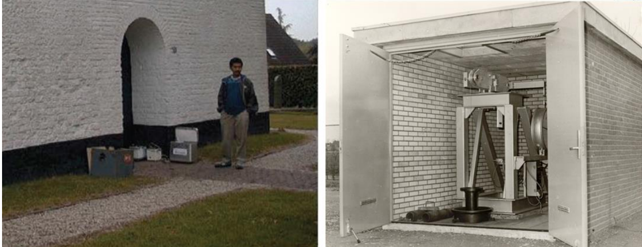
Figure 3: Example of gravity measurement sites used in the 1978-1996 surveys. Left church entrance, right NAM compaction monitoring well – gravity was measured on a cabin floor.
